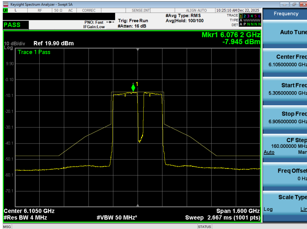
Plot 7-65. In Band Emissions Plot MIMO ANT1 (320MHz 802.11be (3*996+484 Tones) (UNII Band 5) – Ch. 31) VLP
