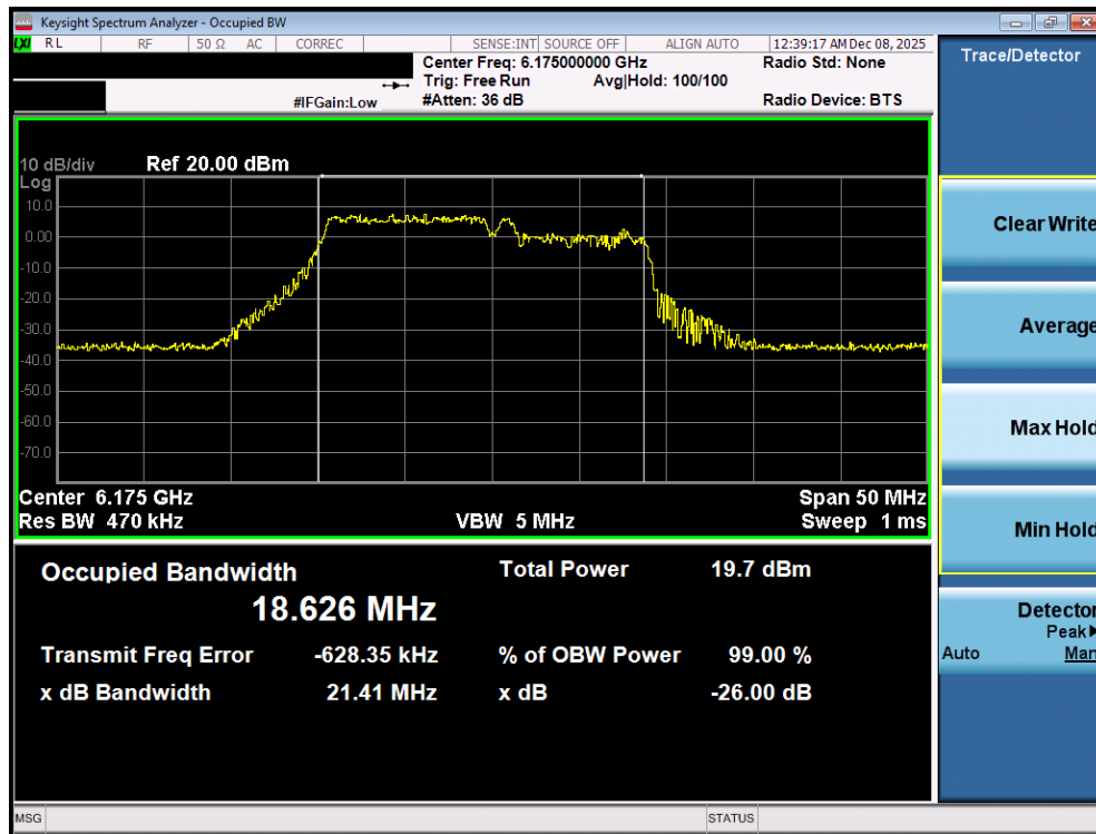
Plot 7-15. 26dB Bandwidth Plot MIMO ANT1 (20MHz 802.11be (106+26 Tones) (UNII Band 5) – Ch. 45) - SP
