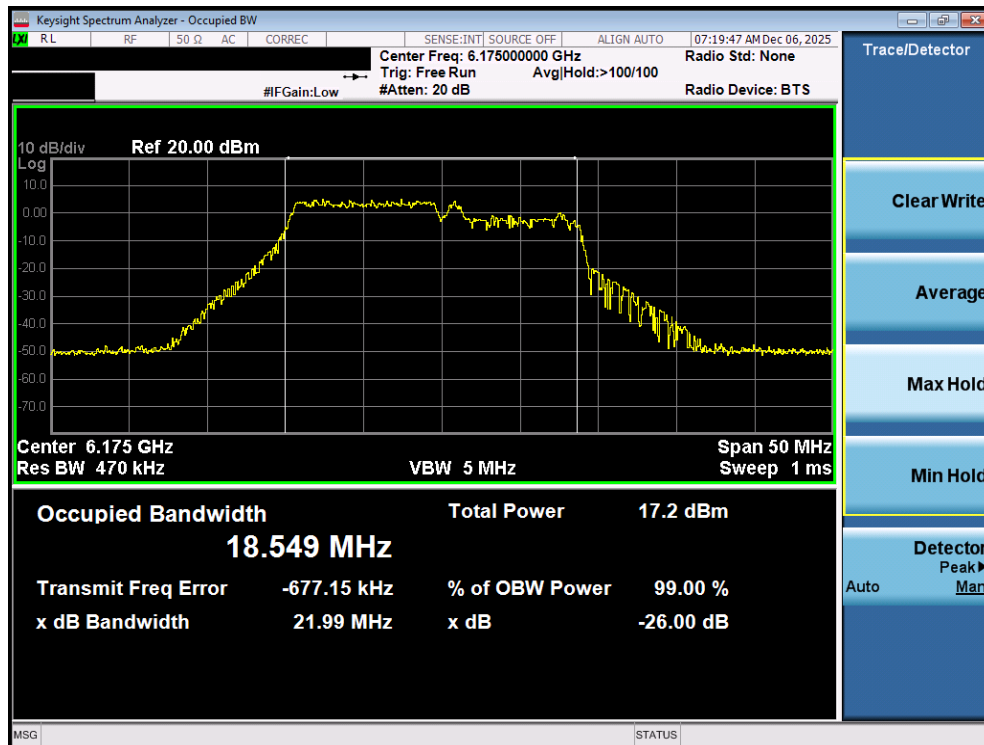
Plot 7-6. 26dB Bandwidth Plot MIMO ANT1 (20MHz 802.11be (106+26 Tones) (UNII Band 5) – Ch. 45) - LPI
