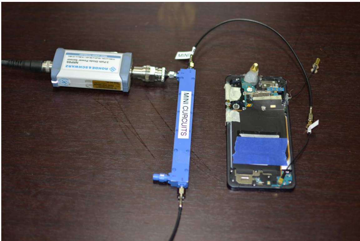
Test Setup Photo 2 – Conducted Test Setup (Figure 5.2-1a)
