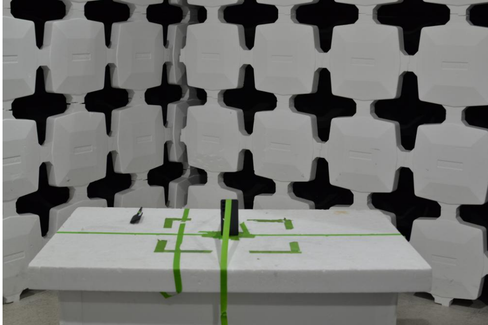
Figure 7. Test Setup – Z Position – 30MHz-1GHz
