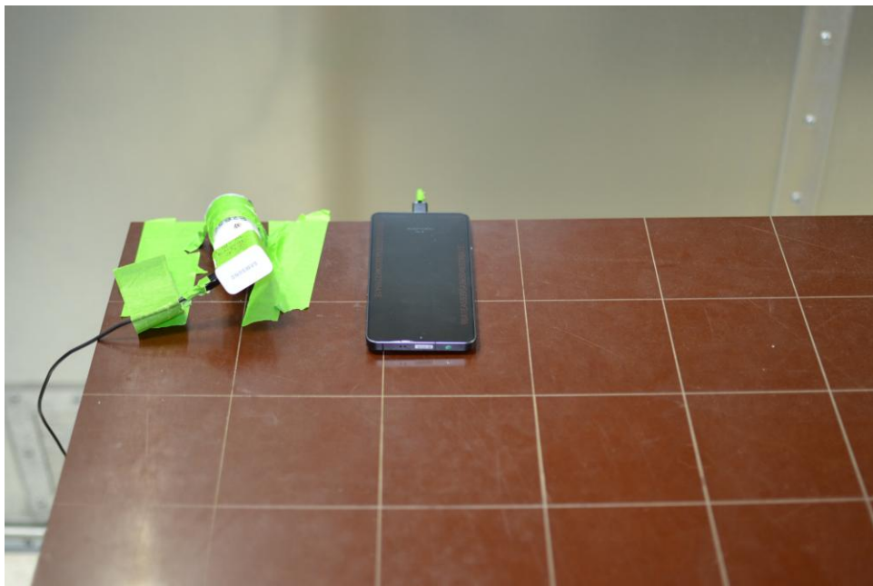
Figure 10. Test Setup – ACLC– <30MHz
