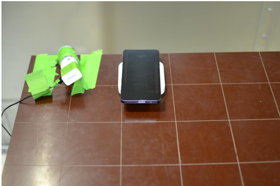
Figure 12. Test Setup – ACLC– <30MHz – with WCP
