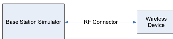
Figure 10-4 Power Measurement Setup – NR FDD
