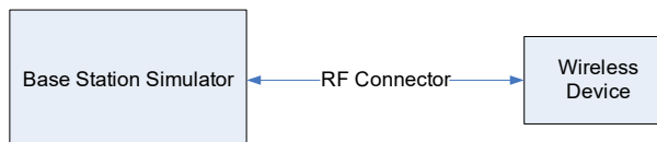
Figure 10-3 Power Measurement Setup
