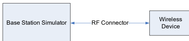
Figure 10-4 Power Measurement Setup – NR FDD
