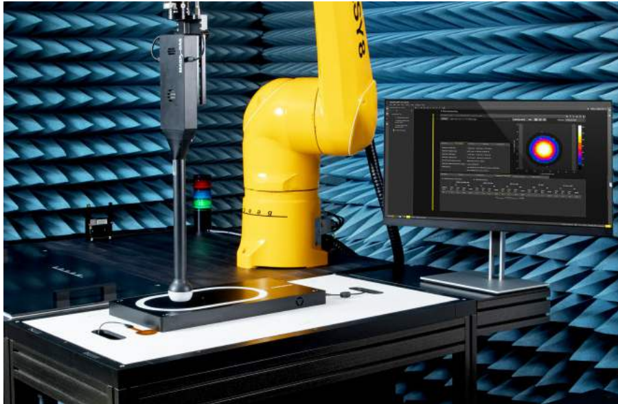
Figure 3-1 DASY 6/8 Module WPT V2.6+ Test System
