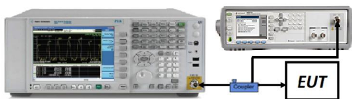
Figure 7-4. Test Instrument & Measurement Setup
