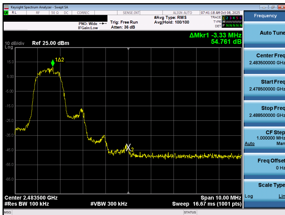
Plot 7-118. Band Edge Plot (Bluetooth with Hopping Disabled, 3 Mbps – Ch. 78) – Dual Ant 1
