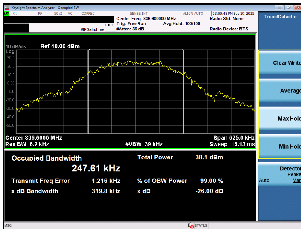
Plot 7-23. Occupied Bandwidth Plot (GPRS, Ch. 190 – Ant1)
