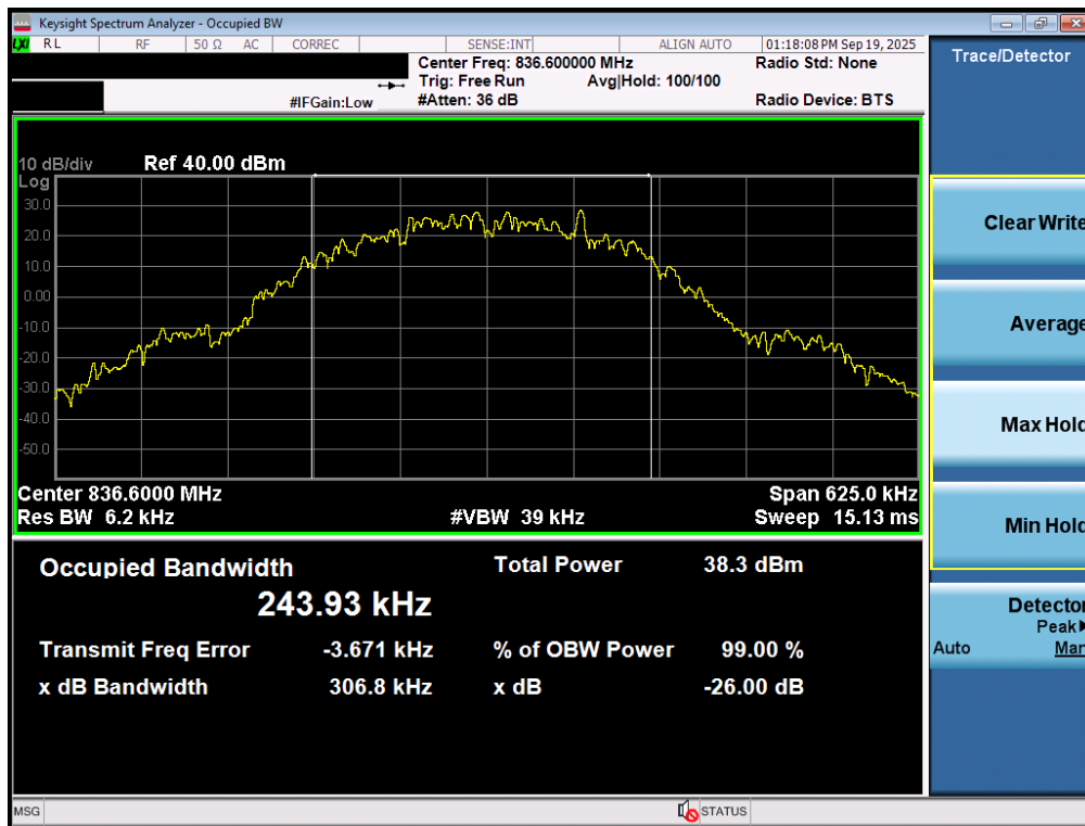
Plot 7-48. Occupied Bandwidth Plot (GPRS, Ch. 190 – Ant2)
