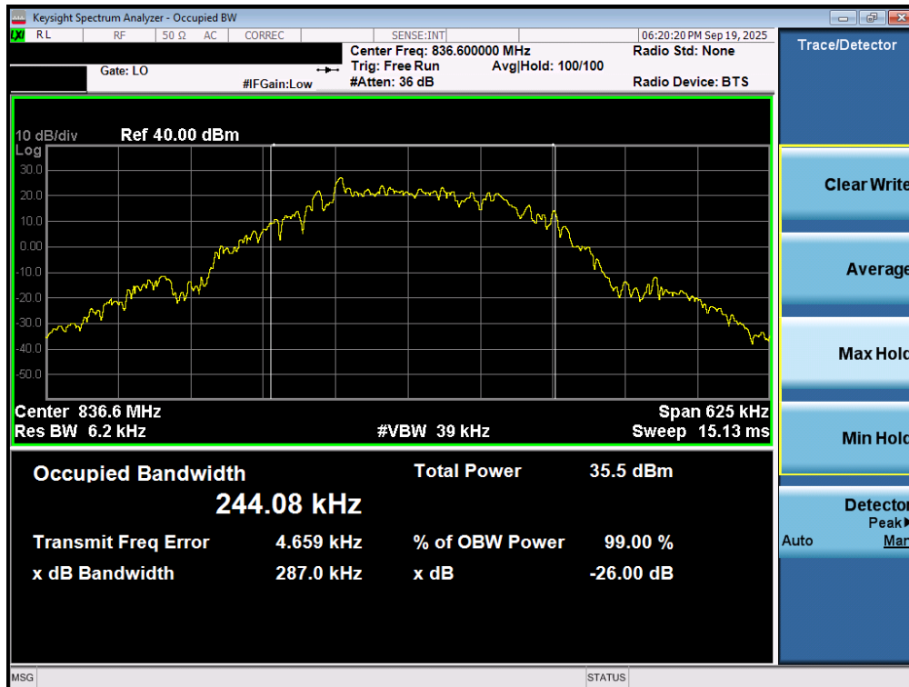
Plot 7-49. Occupied Bandwidth Plot (EDGE, Ch. 190 – Ant2)
