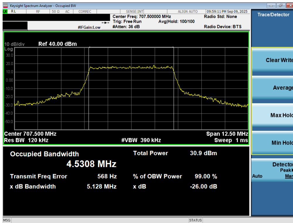
Plot 7-50. Occupied Bandwidth Plot (LTE Band 12/17 - 5MHz 16-QAM - Full RB – ANT2)
