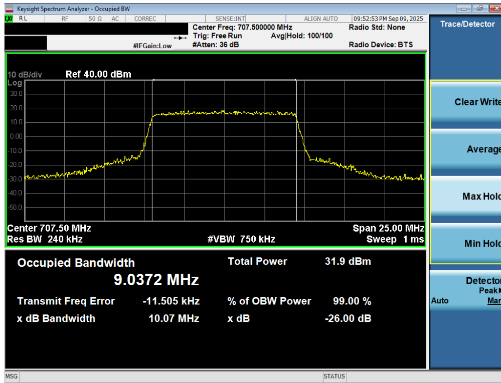
Plot 7-47. Occupied Bandwidth Plot (LTE Band 12/17 - 10MHz QPSK - Full RB – ANT2)
