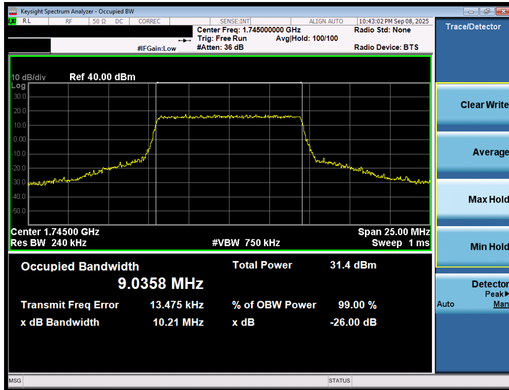
Plot 7-18. Occupied Bandwidth Plot (LTE Band 66/4 - 10MHz QPSK - Full RB - ANT1)
