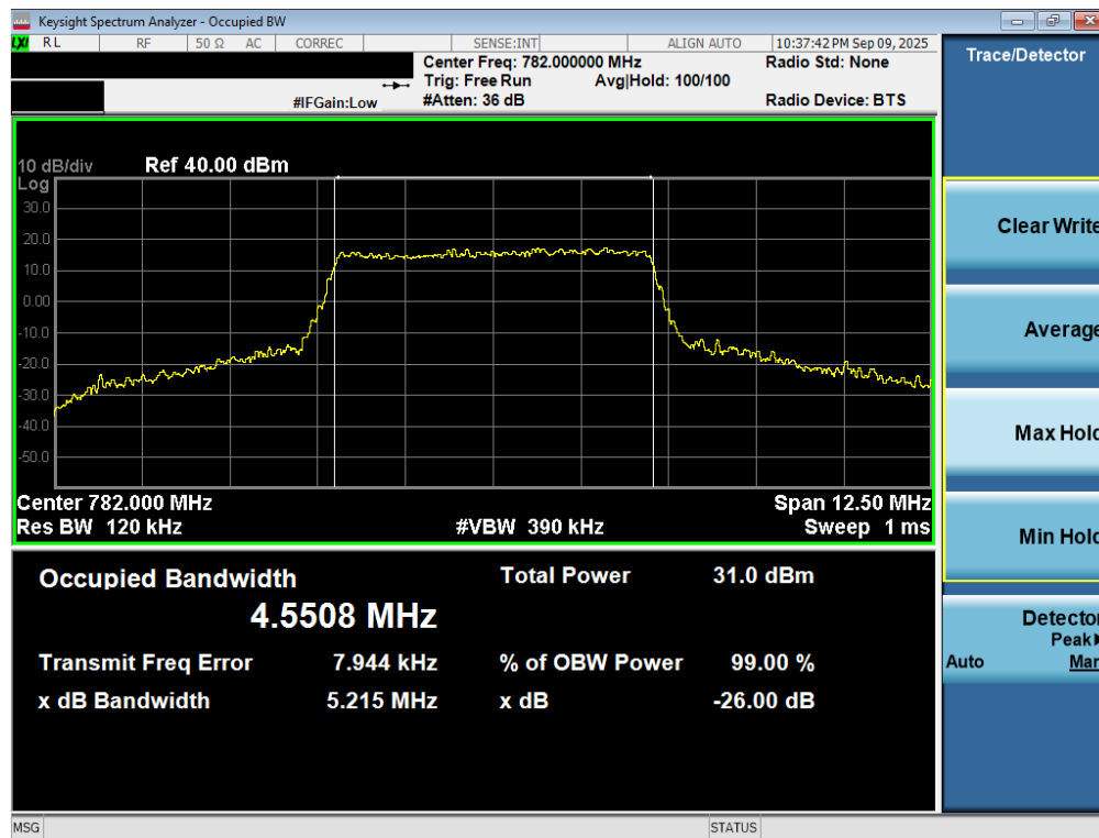
Plot 7-58. Occupied Bandwidth Plot (LTE Band 13 - 5MHz 16-QAM - Full RB – ANT2)
