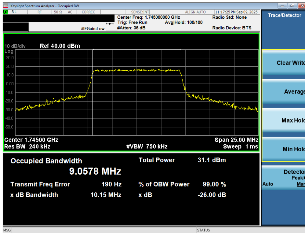
Plot 7-64. Occupied Bandwidth Plot (LTE Band 66/4 - 10MHz 16-QAM - Full RB - ANT2)
