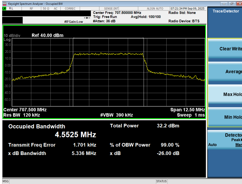
Plot 7-4. Occupied Bandwidth Plot (LTE Band 12/17 - 5MHz QPSK - Full RB – ANT1)
