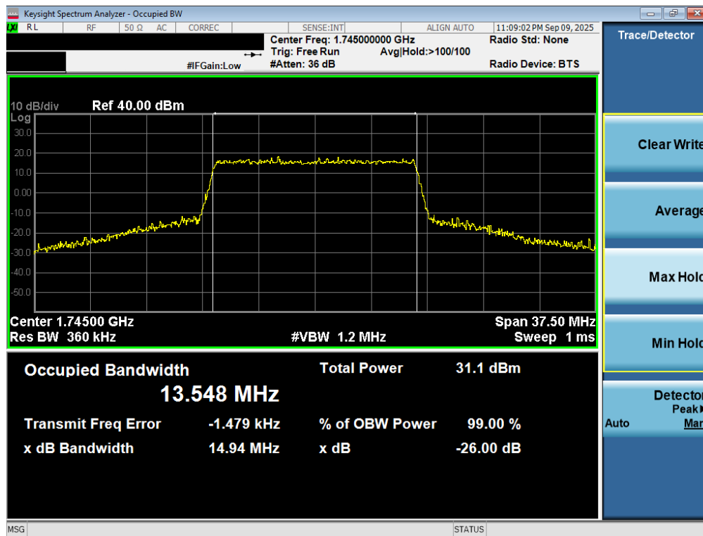
Plot 7-62. Occupied Bandwidth Plot (LTE Band 66/4 - 15MHz 16-QAM - Full RB - ANT2)
