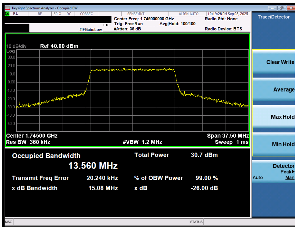
Plot 7-17. Occupied Bandwidth Plot (LTE Band 66/4 - 15MHz 16-QAM - Full RB - ANT1)
