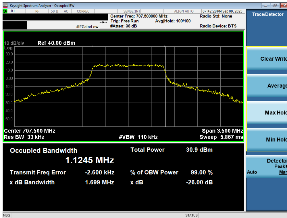
Plot 7-9. Occupied Bandwidth Plot (LTE Band 12/17 – 1.4MHz 16-QAM - Full RB – ANT1)
