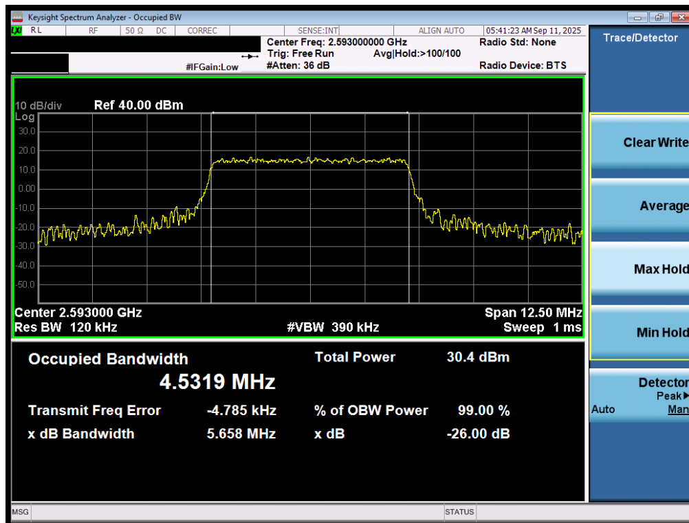
Plot 7-116. Occupied Bandwidth Plot (LTE Band 41(PC3) - 5MHz 16-QAM - Full RB - Ant2)
