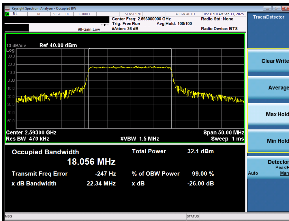
Plot 7-109. Occupied Bandwidth Plot (LTE Band 41(PC3) - 20MHz QPSK - Full RB - Ant2)
