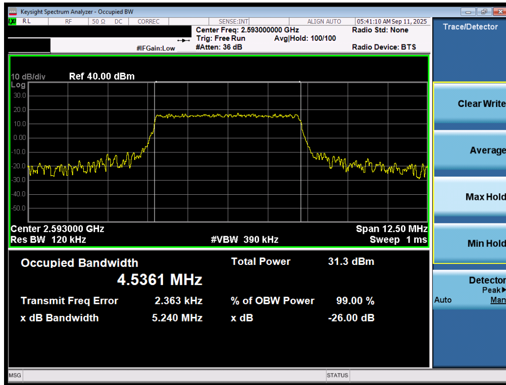
Plot 7-115. Occupied Bandwidth Plot (LTE Band 41(PC3) - 5MHz QPSK - Full RB - Ant2)
