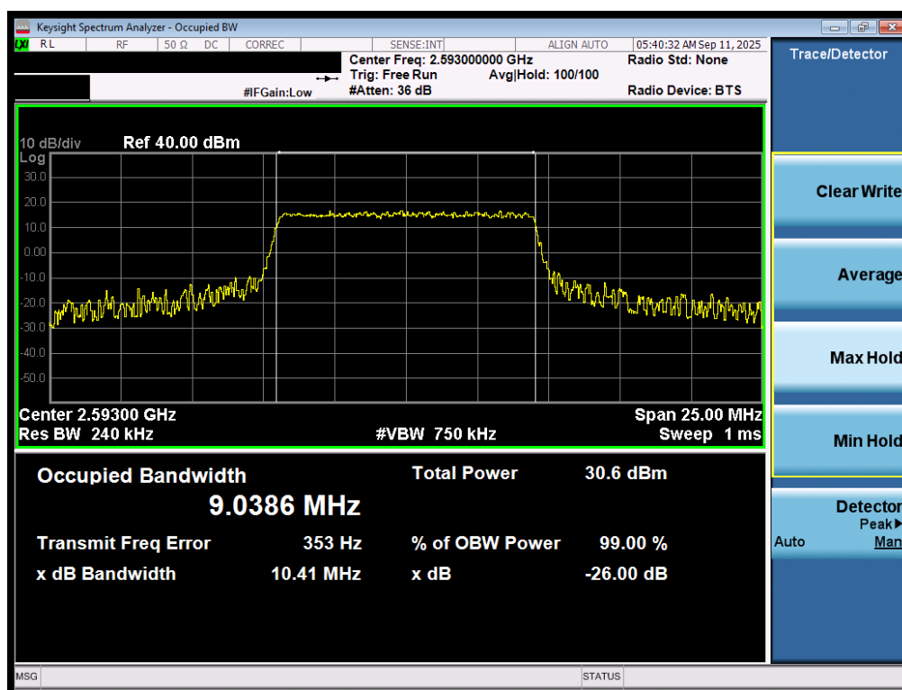
Plot 7-114. Occupied Bandwidth Plot (LTE Band 41(PC3) - 10MHz 16-QAM - Full RB - Ant2)
