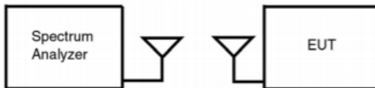
Figure 7-1. Test Instrument and Measurement Setup
