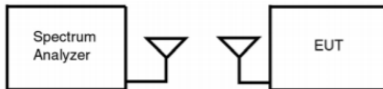
Figure 7-2. Test Instrument and Measurement Setup
