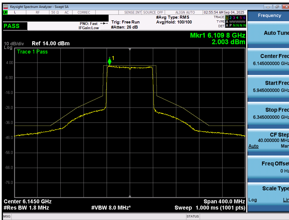
Plot 7-73. In Band Emissions Plot MIMO ANT1 (80MHz 802.11ax/be (UNII Band 5) – Ch. 39) – SP
