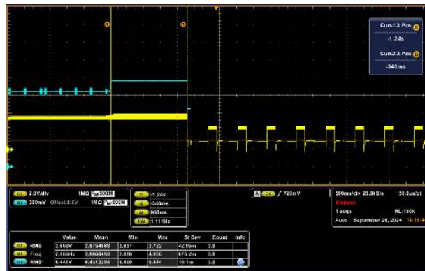
Figure 2-1 WPT Load Removal Power Down
