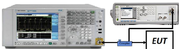
Figure 7-1. Test Instrument & Measurement Setup
