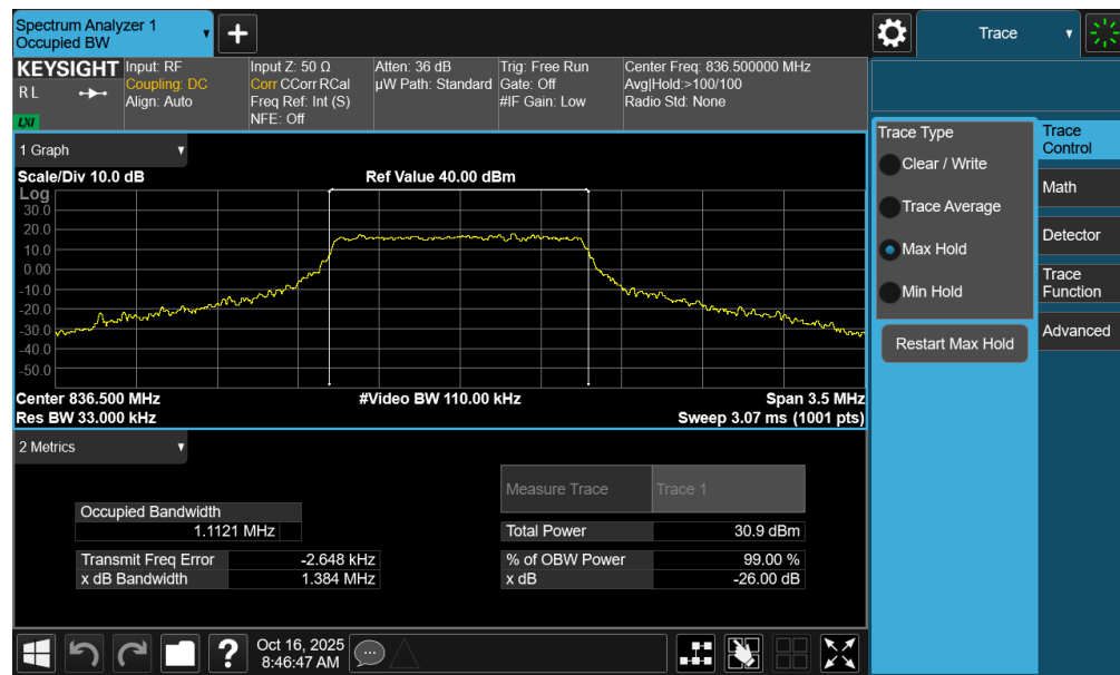
Plot 7-8. Occupied Bandwidth Plot (LTE Band 5 - 1.4MHz 16-QAM - Full RB - Ant1)
