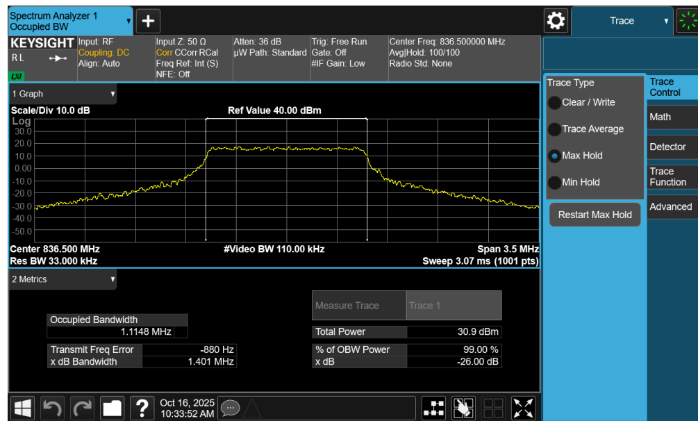
Plot 7-31. Occupied Bandwidth Plot (LTE Band 5 - 1.4MHz 16-QAM - Full RB - Ant2)
