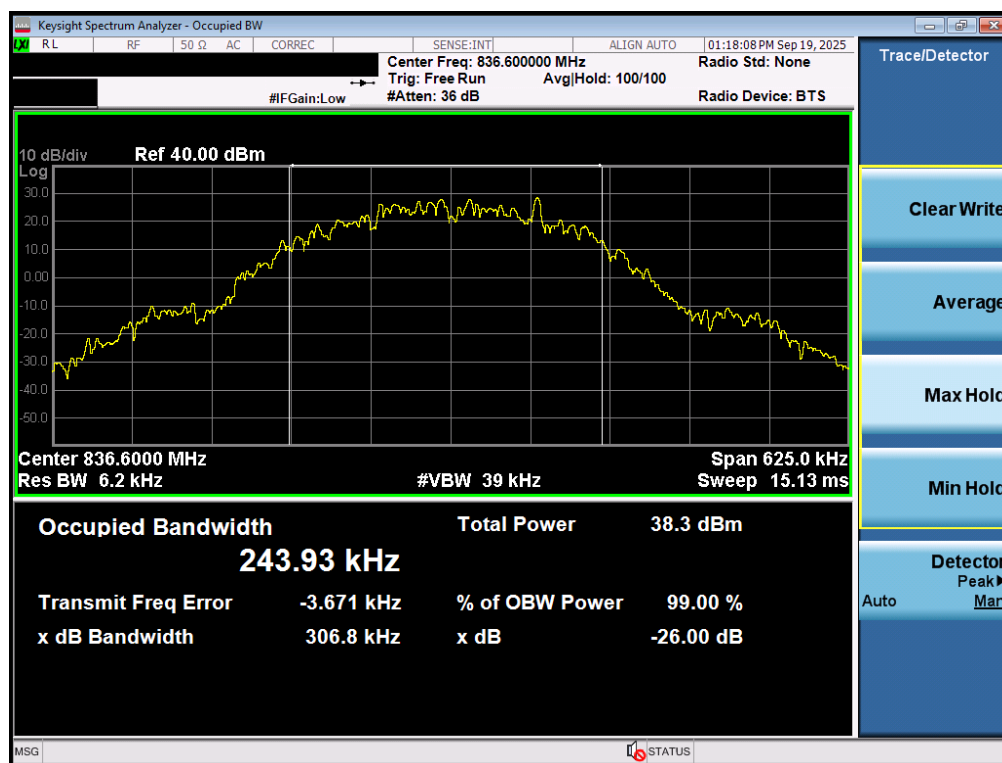
Plot 7-44. Occupied Bandwidth Plot (GPRS, Ch. 190 – Ant2)
