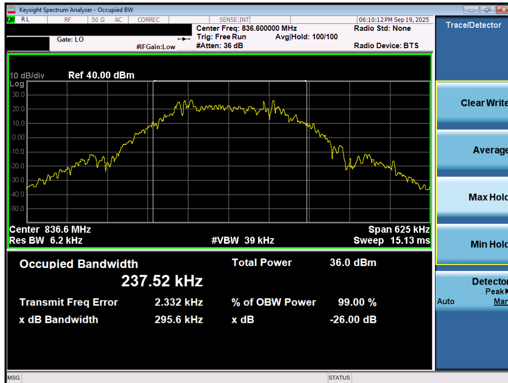
Plot 7-22. Occupied Bandwidth Plot (EDGE, Ch. 190 – Ant1)
