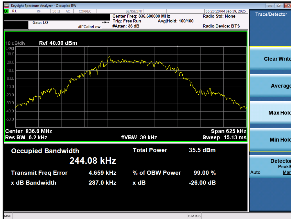
Plot 7-45. Occupied Bandwidth Plot (EDGE, Ch. 190 – Ant2)
