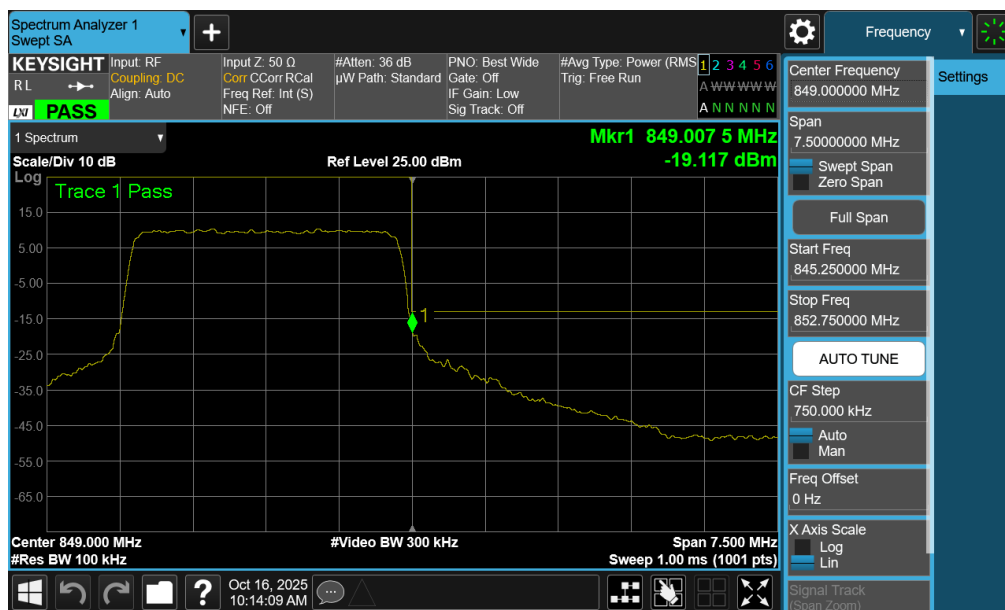
Plot 7-124. Upper Band Edge Plot (LTE Band 5 - 3MHz QPSK – Full RB - Ant1)
