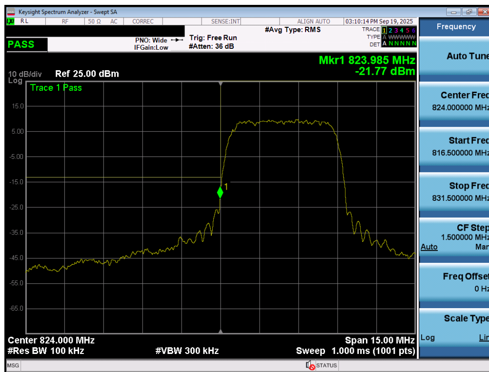
Plot 7-137. Lower Band Edge Plot (WCDMA Cell – Ch. 4132 – Ant1)
