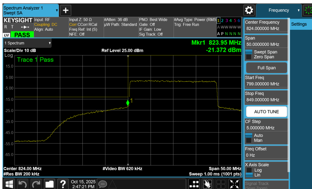
Plot 7-147. Lower Band Edge Plot (NR Band n5 – 20.0MHz - Full RB - Ant2)
