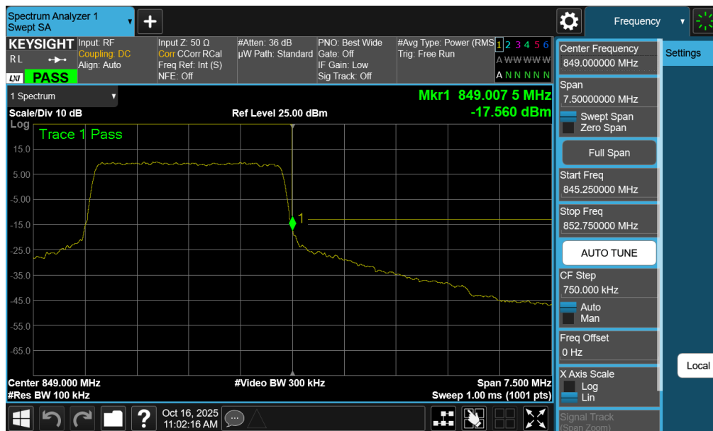
Plot 7-144. Upper Band Edge Plot (LTE Band 5 - 3MHz QPSK – Full RB - Ant2)
