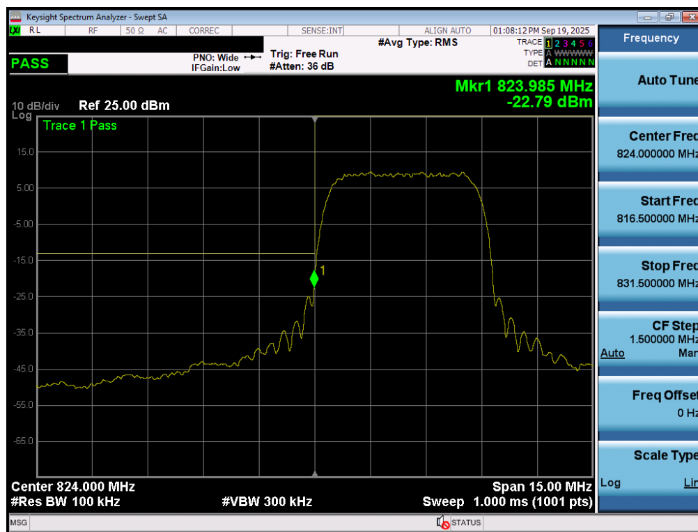
Plot 7-157. Lower Band Edge Plot (WCDMA Cell – Ch. 4132 – Ant2)
