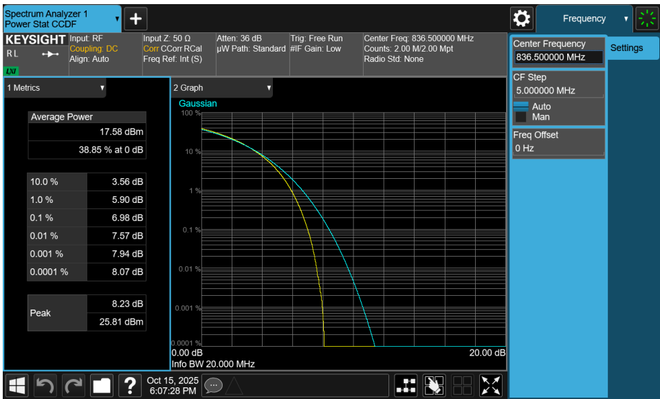
Plot 7-166. Peak-Average Ratio Plot (NR Band n5 - 20MHz 256-QAM - Full RB - Ant1)
