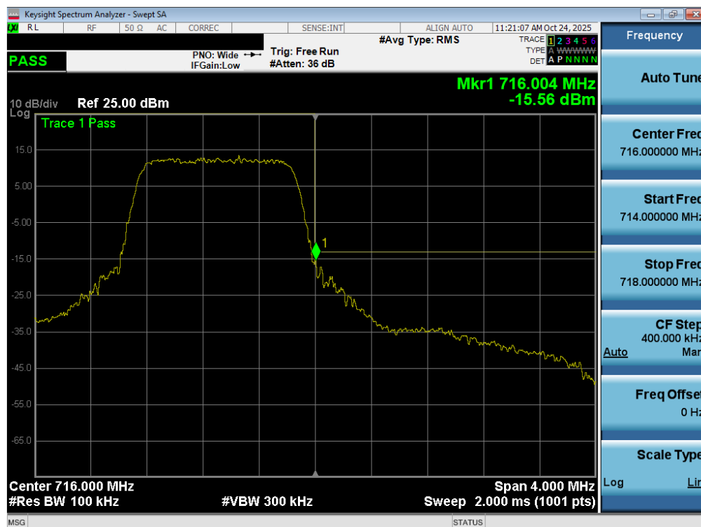
Plot 7-129. Upper Band Edge Plot (LTE Band 12 – 1.4MHz QPSK – Full RB - ANT2)
