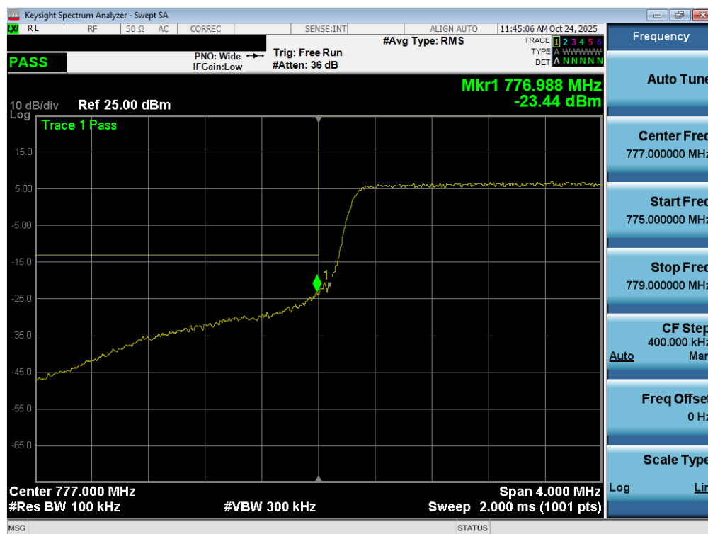
Plot 7-130. Lower Band Edge Plot (LTE Band 13 - 5MHz QPSK – Full RB - ANT2)
