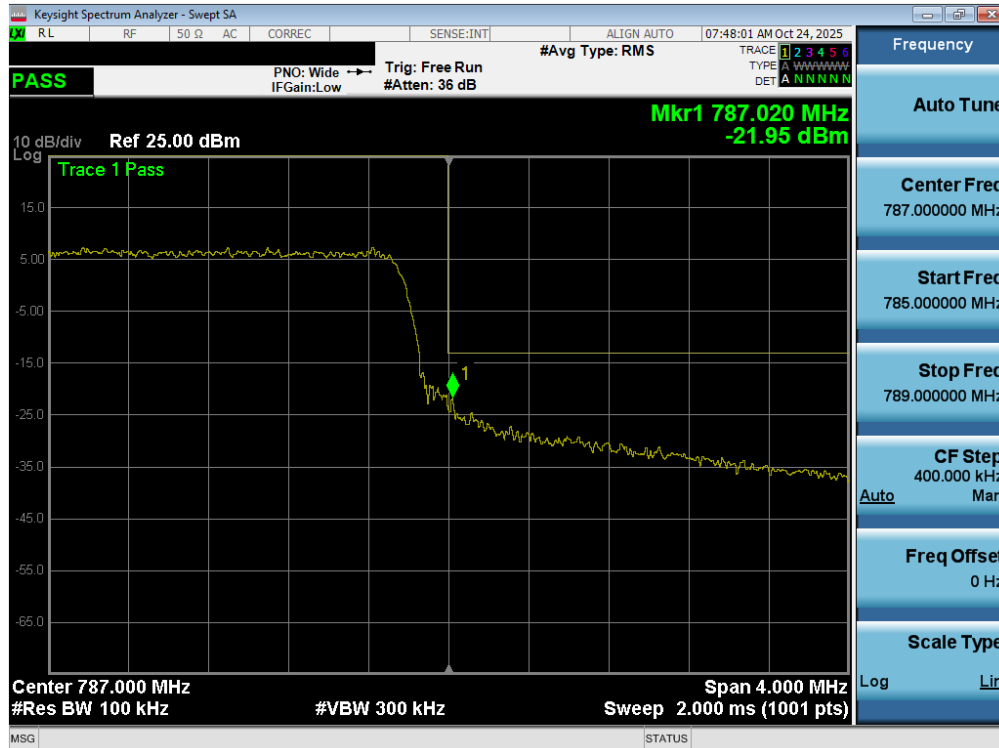
Plot 7-116. Upper Band Edge Plot (LTE Band 13 - 5MHz QPSK – Full RB - ANT1)
