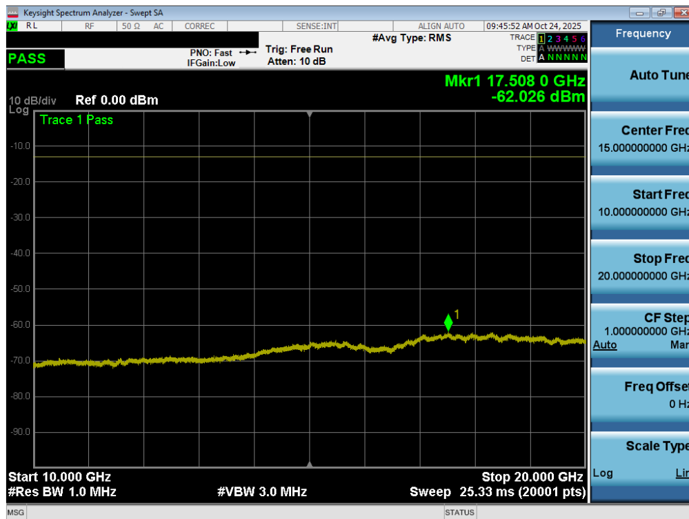
Plot 7-99. Conducted Spurious Plot (LTE Band 66/4 - 20MHz QPSK - 1 RB – Mid Channel)
