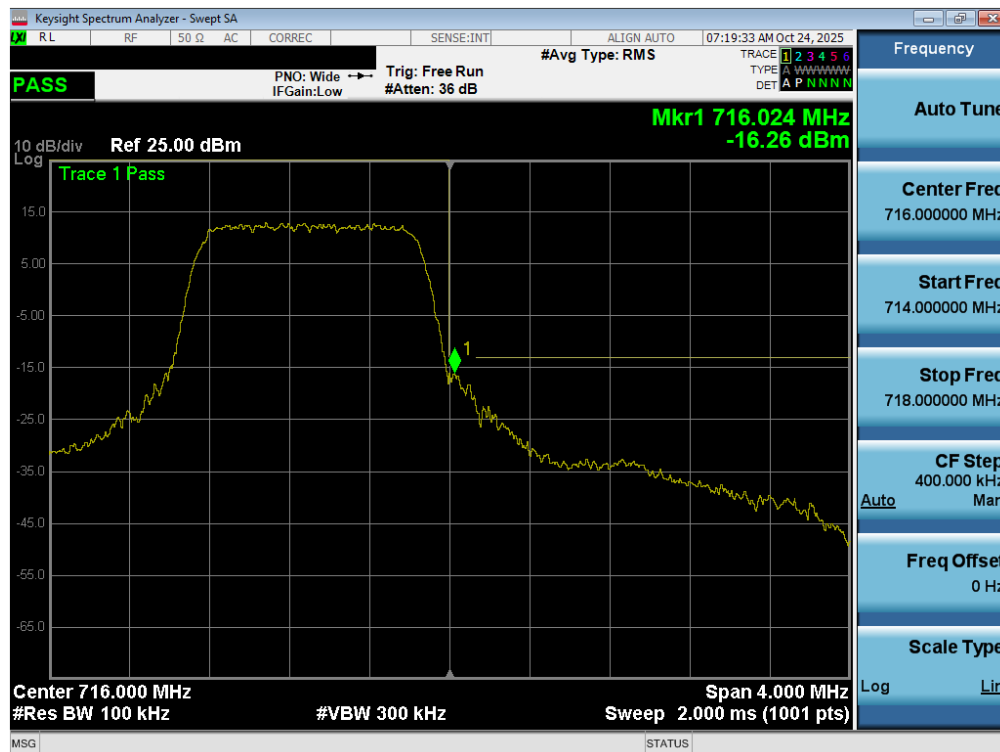
Plot 7-113. Upper Band Edge Plot (LTE Band 12 – 1.4MHz QPSK – Full RB - ANT1)
