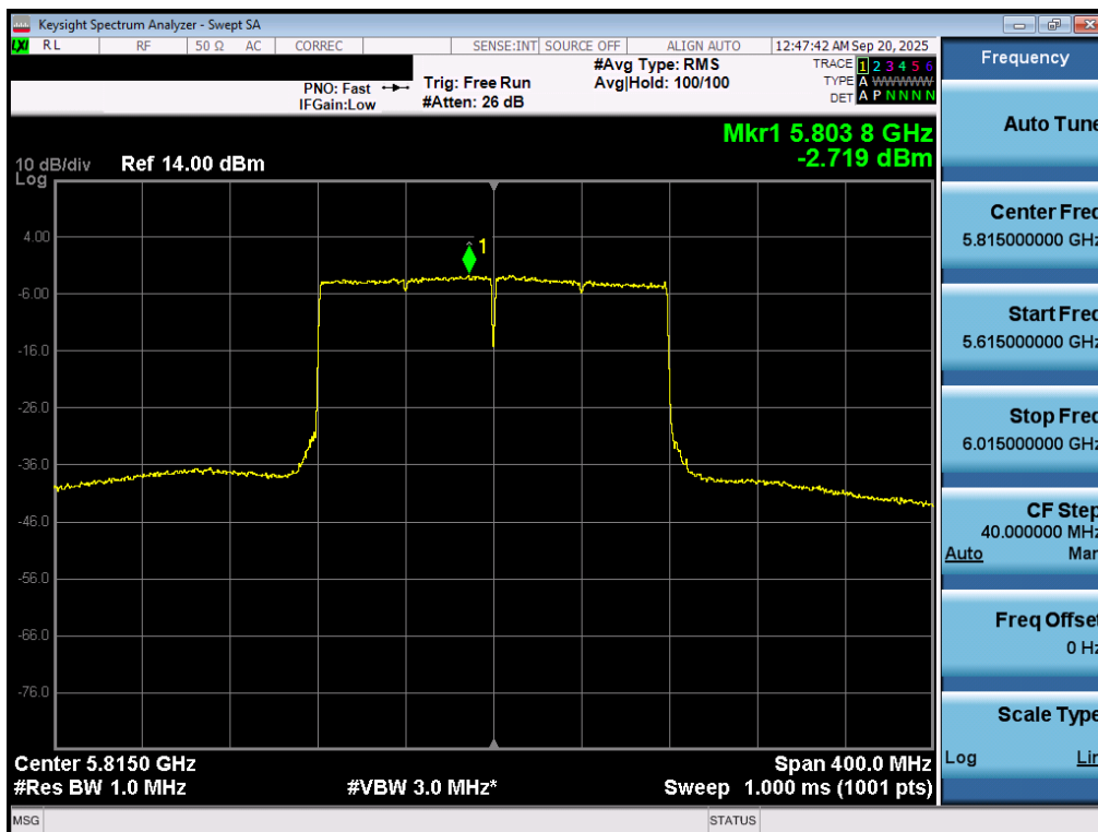
Plot 7-88. Power Spectral Density Plot MIMO ANT1 (160MHz BW 802.11be (UNII Band 3/4) – Ch. 163)
