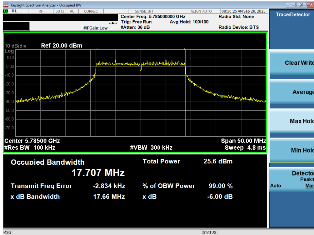
Plot 7-43. 6dB Bandwidth Plot MIMO ANT2 (20MHz BW 802.11n (UNII Band 3) – Ch. 157)
