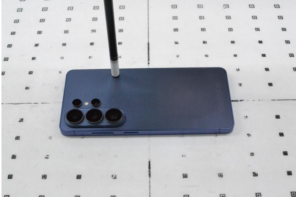
PD Test Setup Photo 27 – PD, Back Side at 2mm (Antenna H)
