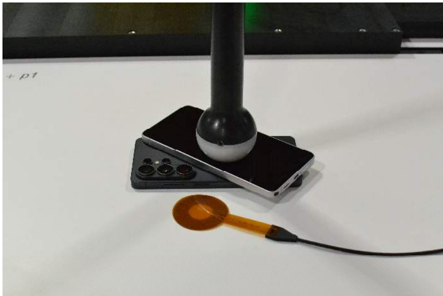
Test Setup Photo 8 Device to Device - Offset, Back Side, 0mm
