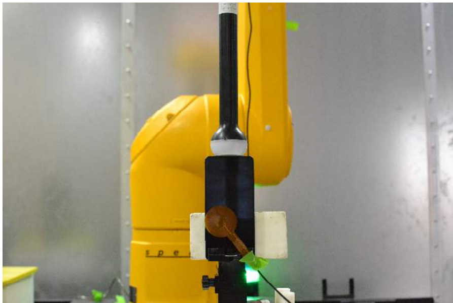
Test Setup Photo 4 Standby (Ping) Signal, Bottom Side, 0mm
