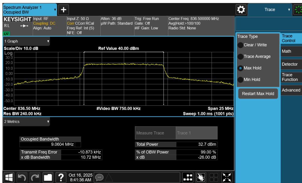
Plot 7-3. Occupied Bandwidth Plot (LTE Band 26/5 - 10MHz QPSK - Full RB - Ant1)
