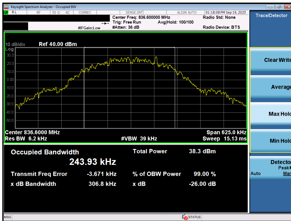
Plot 7-48. Occupied Bandwidth Plot (GPRS, Ch. 190 – Ant2)
