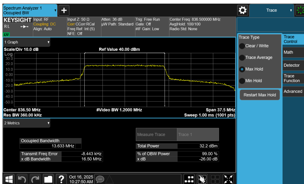
Plot 7-26. Occupied Bandwidth Plot (LTE Band 26 - 15MHz QPSK - Full RB - Ant2)
