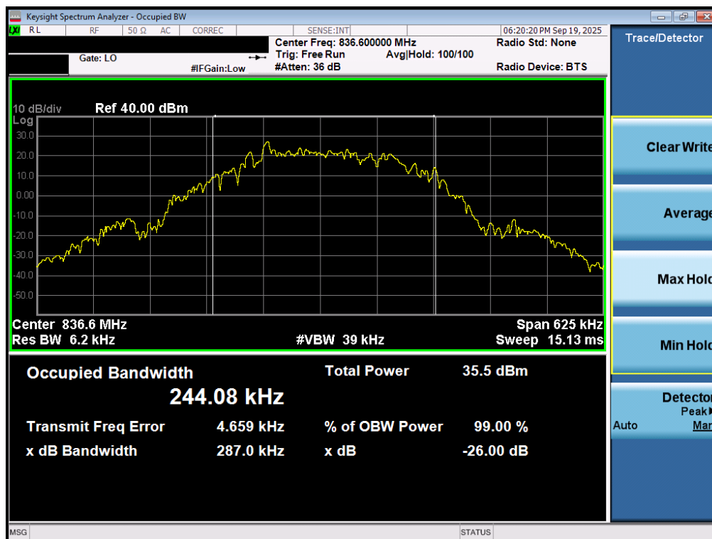
Plot 7-49. Occupied Bandwidth Plot (EDGE, Ch. 190 – Ant2)
