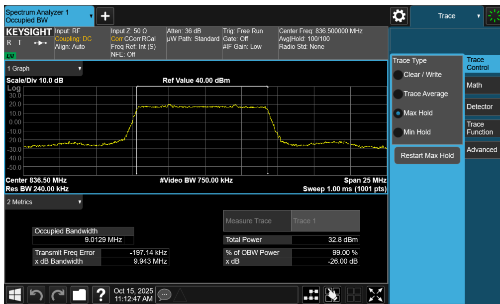
Plot 7-17. Occupied Bandwidth Plot (NR Band n26/5 - 10MHz \pi/2 BPSK - Full RB - Ant1)
