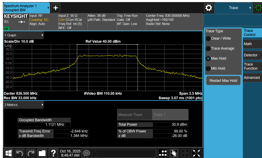
Plot 7-10. Occupied Bandwidth Plot (LTE Band 26/5 - 1.4MHz 16-QAM - Full RB - Ant1)
