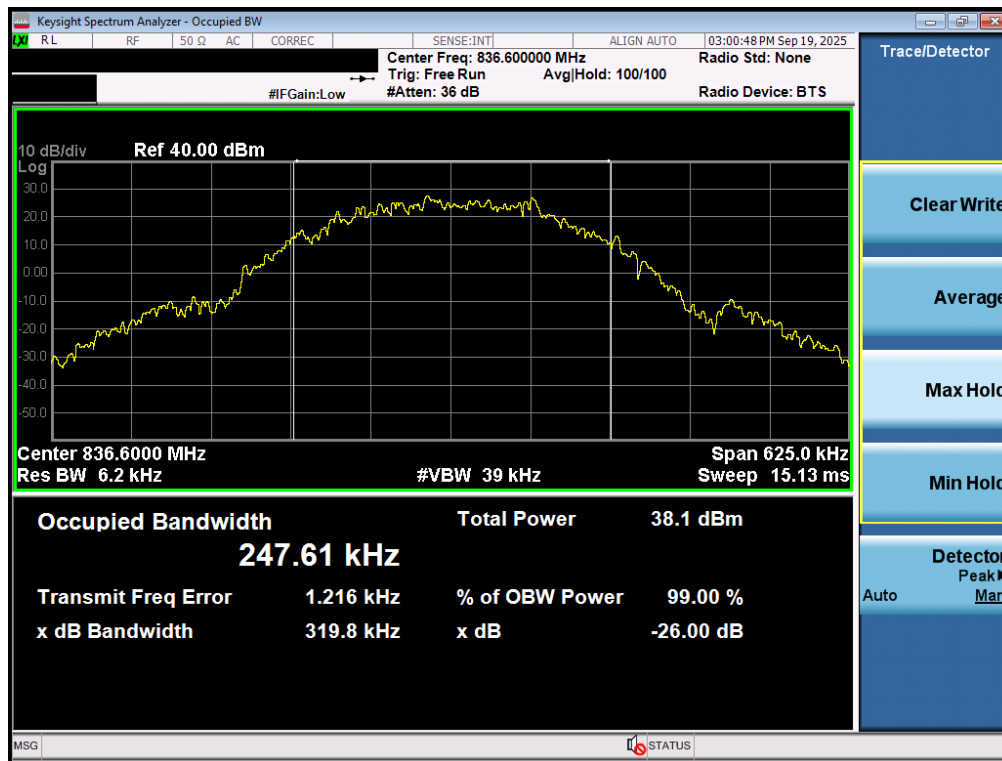
Plot 7-23. Occupied Bandwidth Plot (GPRS, Ch. 190 – Ant1)
