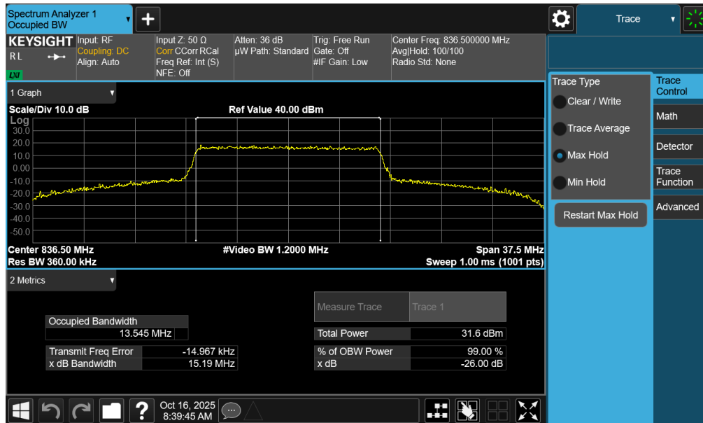
Plot 7-2. Occupied Bandwidth Plot (LTE Band 26 - 15MHz 16-QAM - Full RB - Ant1)
