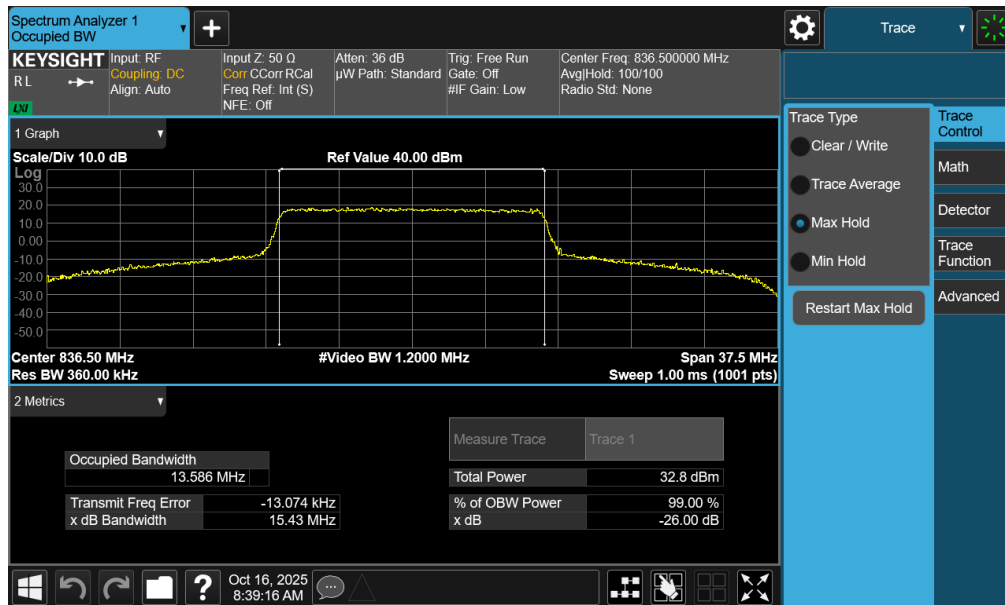
Plot 7-1. Occupied Bandwidth Plot (LTE Band 26 - 15MHz QPSK - Full RB - Ant1)
