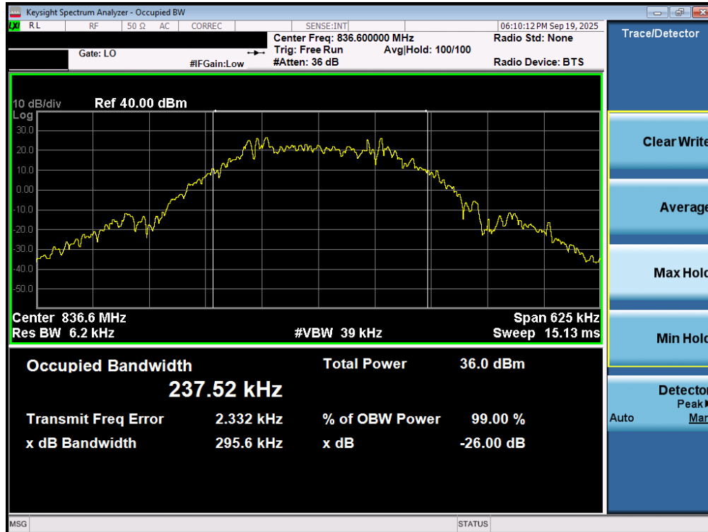
Plot 7-24. Occupied Bandwidth Plot (EDGE, Ch. 190 – Ant1)
