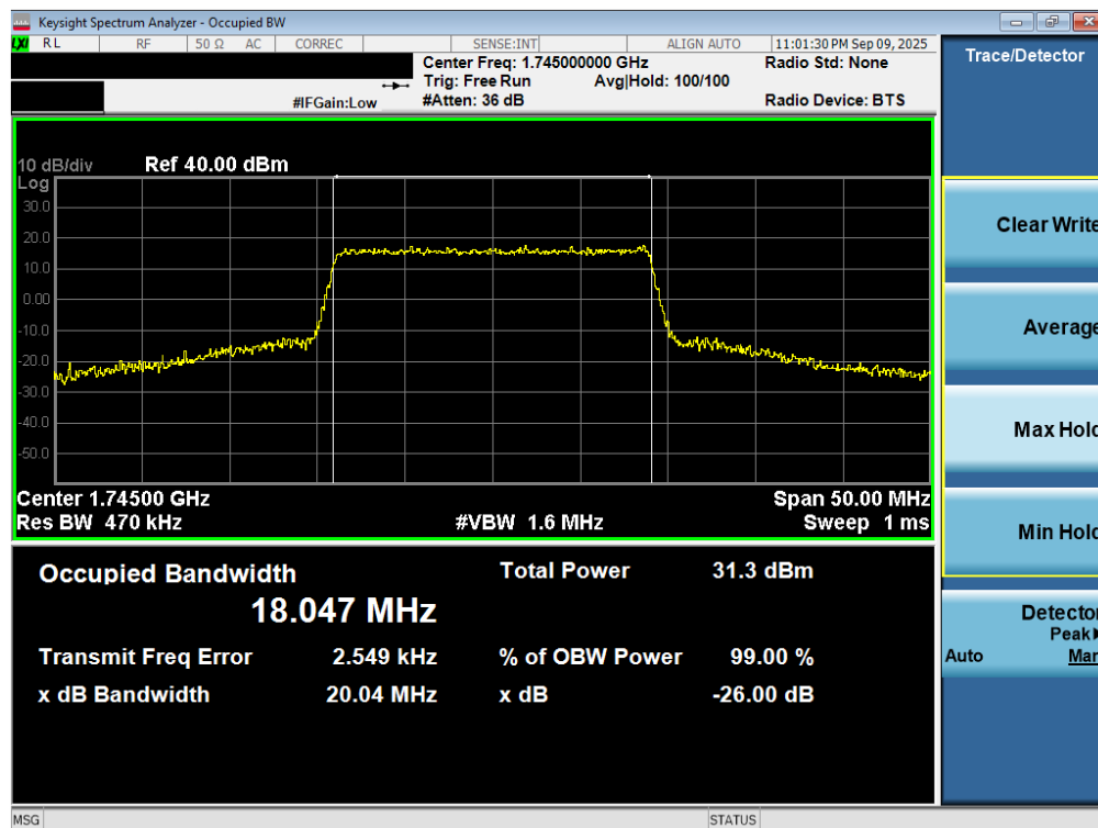
Plot 7-121. Occupied Bandwidth Plot (LTE Band 66/4 - 20MHz 16-QAM - Full RB - ANT2)
