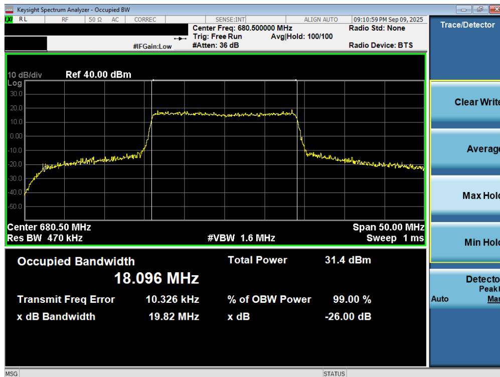
Plot 7-101. Occupied Bandwidth Plot (LTE Band 71 - 20MHz 16-QAM - Full RB – ANT2)
