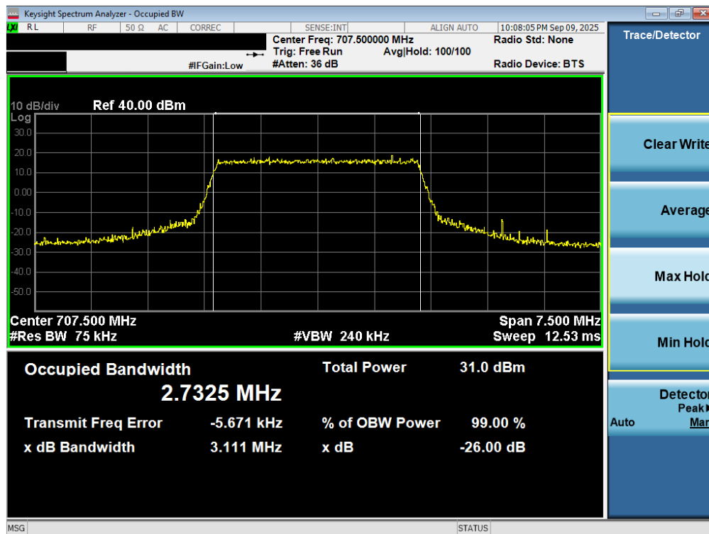
Plot 7-113. Occupied Bandwidth Plot (LTE Band 12 - 3MHz 16-QAM - Full RB – ANT2)
