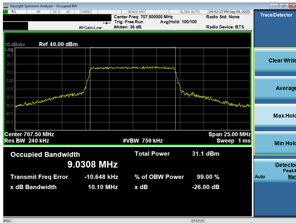
Plot 7-109. Occupied Bandwidth Plot (LTE Band 12 - 10MHz 16-QAM - Full RB – ANT2)
