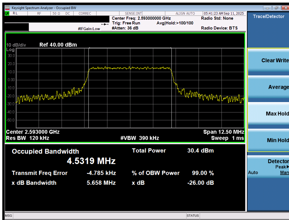
Plot 7-155. Occupied Bandwidth Plot (LTE Band 41(PC3)/38 - 5MHz 16-QAM - Full RB - Ant2)
