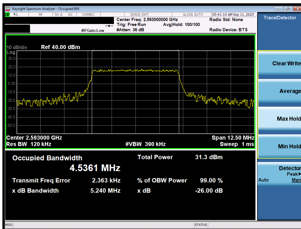
Plot 7-154. Occupied Bandwidth Plot (LTE Band 41(PC3)/38 - 5MHz QPSK - Full RB - Ant2)
