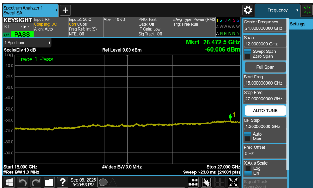
Plot 7-205. Conducted Spurious Plot (LTE Band 7 - 20MHz QPSK - RB Size 1, RB Offset 0 - High Channel - Ant1)
