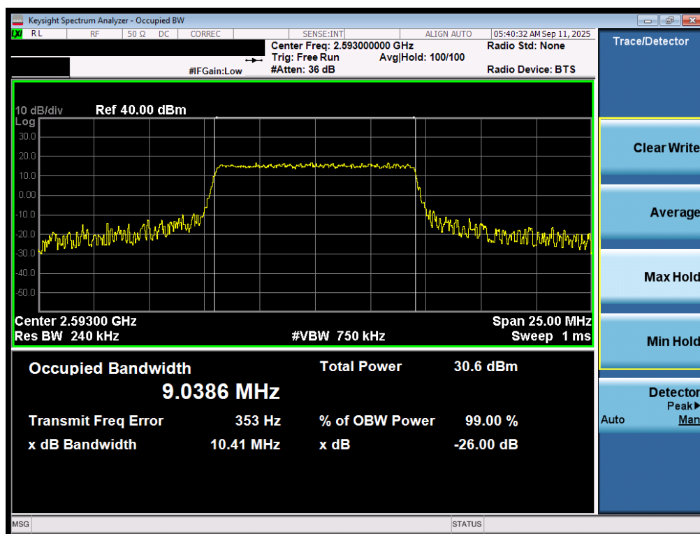
Plot 7-153. Occupied Bandwidth Plot (LTE Band 41(PC3)/38 - 10MHz 16-QAM - Full RB - Ant2)
