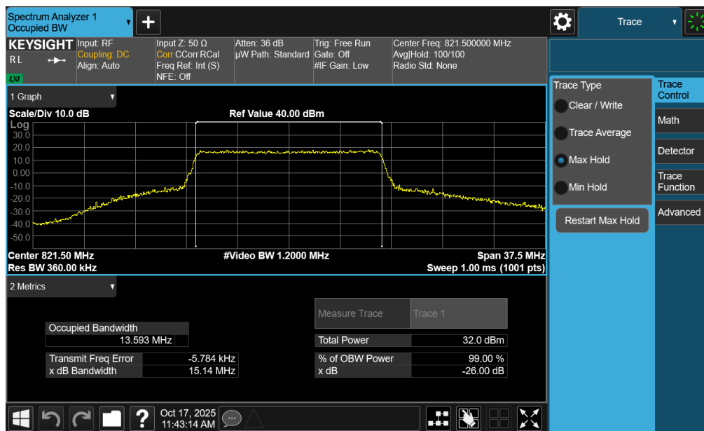
Plot 7-49. Occupied Bandwidth Plot (LTE Band 26 - 15MHz 16-QAM - Full RB)
