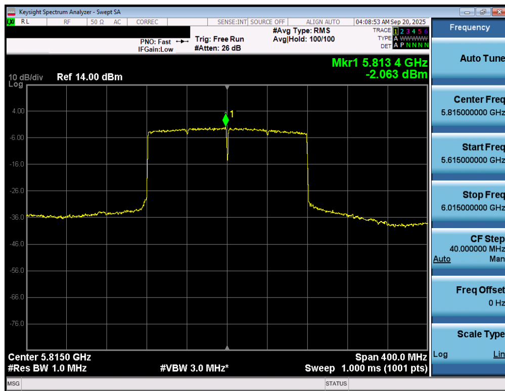
Plot 7-76. Power Spectral Density Plot MIMO ANT1 (160MHz BW 802.11be – 996*2 Tones (UNII Band 3/4) – Ch. 163)
