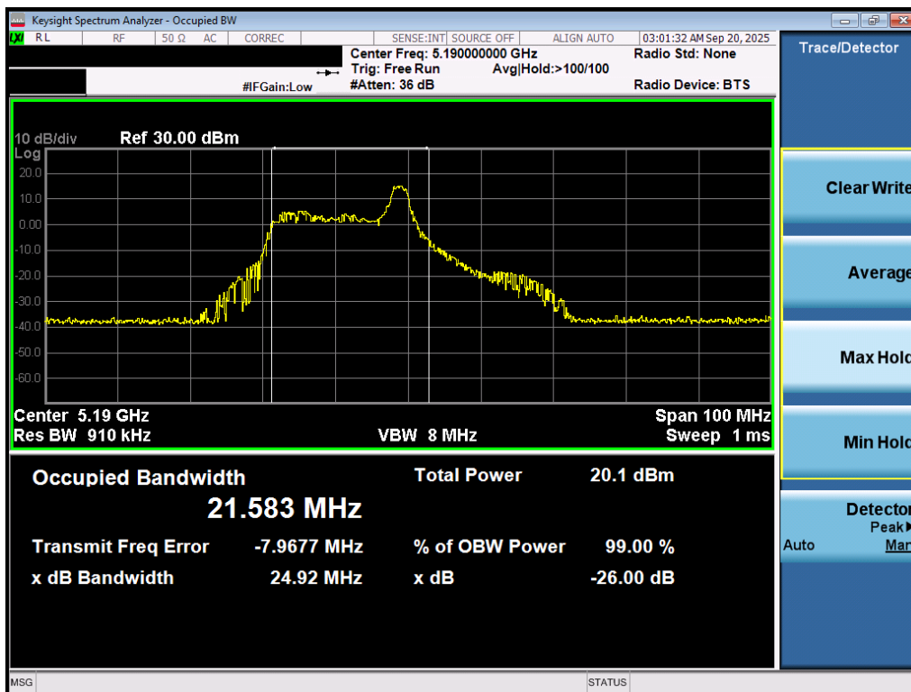
Plot 7-2. 26dB Bandwidth Plot MIMO ANT1 (40MHz BW 802.11be – 26 Tones (UNII Band 1) – Ch. 38)
