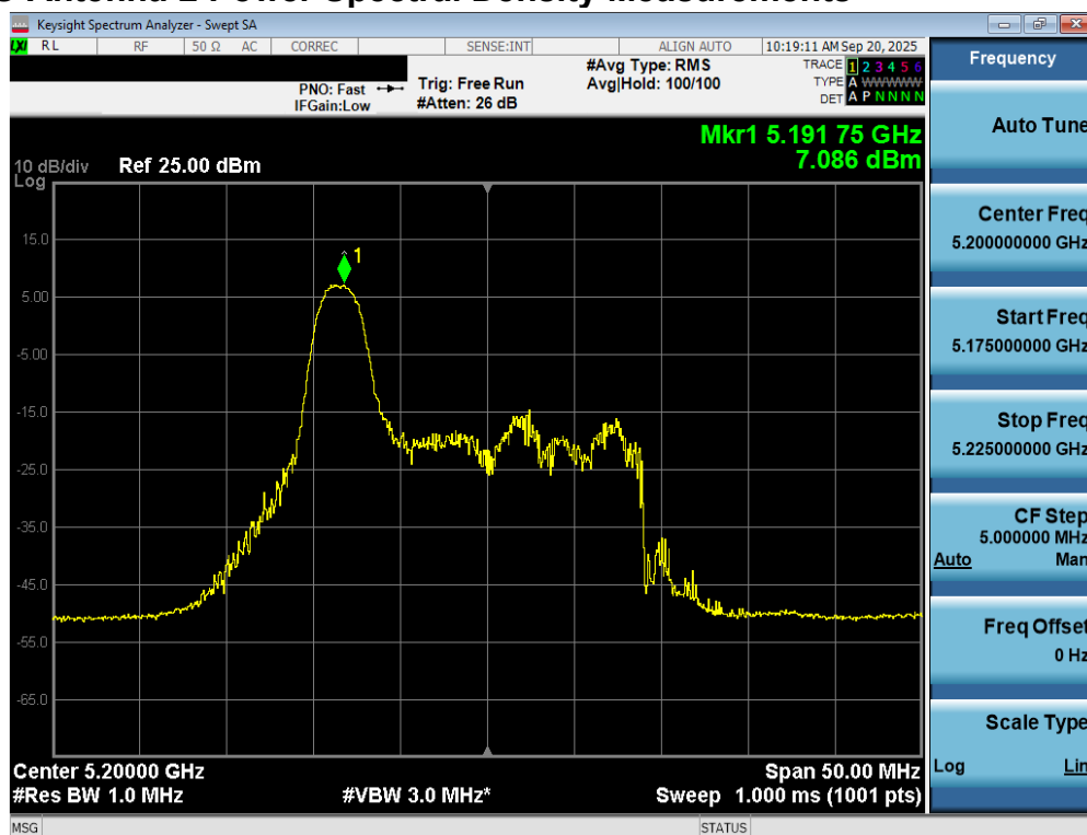
Plot 7-82. Power Spectral Density Plot MIMO ANT2 (20MHz BW 802.11be – 26 Tones (UNII Band 1) – Ch. 40)
