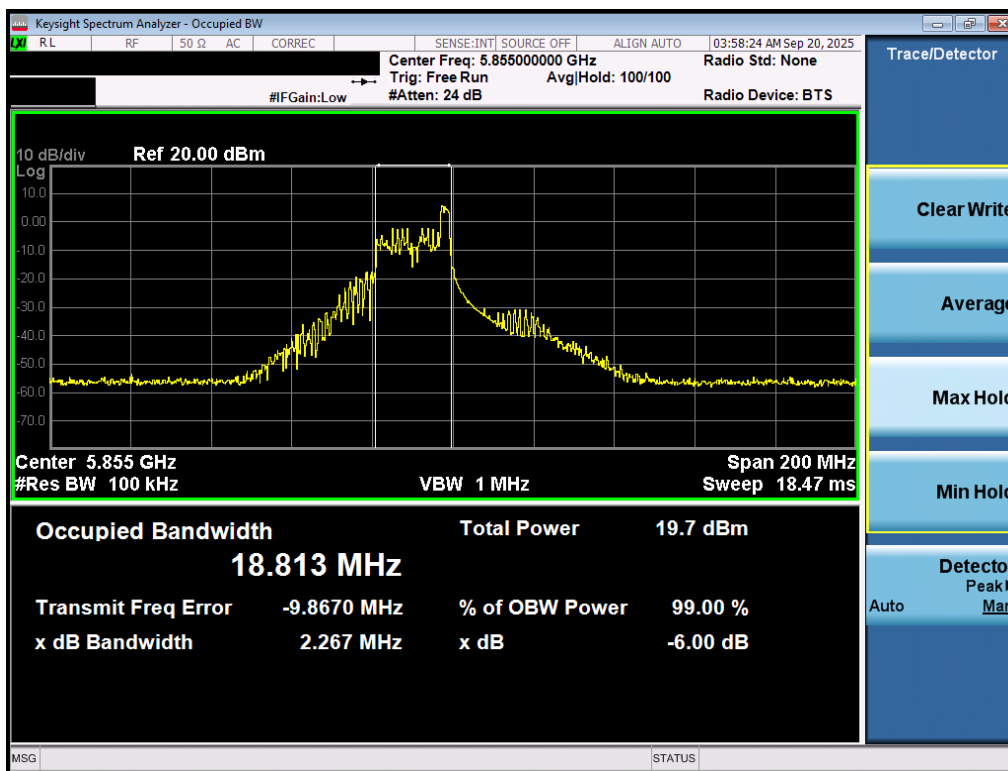
Plot 7-26. 6dB Bandwidth Plot MIMO ANT1 (80MHz BW 802.11be – 26 Tones (UNII Band 3/4) – Ch. 171)
