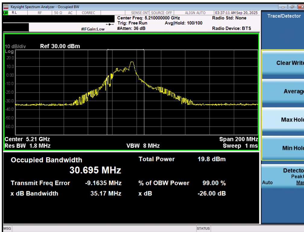
Plot 7-3. 26dB Bandwidth Plot MIMO ANT1 (80MHz BW 802.11be – 26 Tones (UNII Band 1) – Ch. 42)
