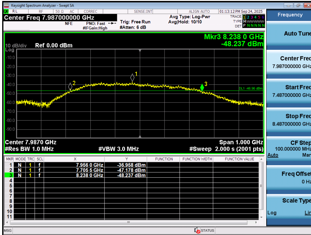
Plot 7-27. 10dBc Bandwidth – CH.9 – SP3 – Preamble 12
