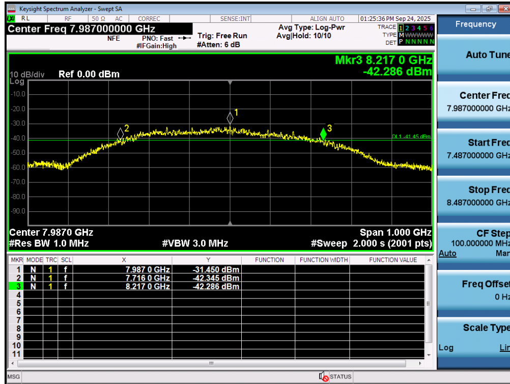
Plot 7-29. 10dBc Bandwidth – CH.9 – SP1 – Preamble 27
