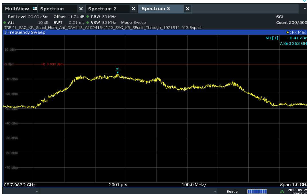
Plot 7-33. UWB Peak Power Measurement - CH.9 – BPRF
