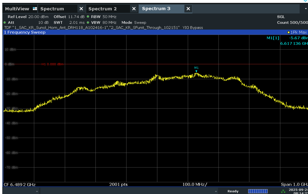
Plot 7-32. UWB Peak Power Measurement - CH.5 – BPRF
