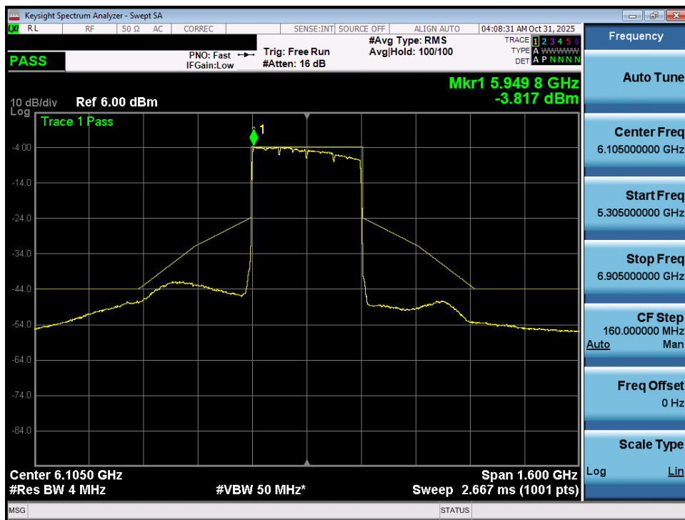
Plot 7-70. In Band Emissions Plot MIMO ANT1 (320MHz 802.11be (Full Tones) (UNII Band 5) – Ch. 31) - VLP
