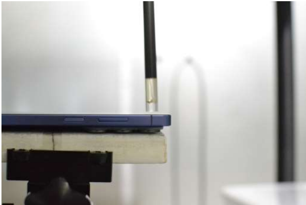
Figure 18-2 Test Setup for Wireless Device – Single Point Measurement
