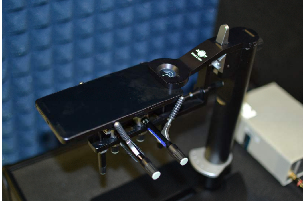
Figure 17-1 Wireless Device in Handset Positioner
