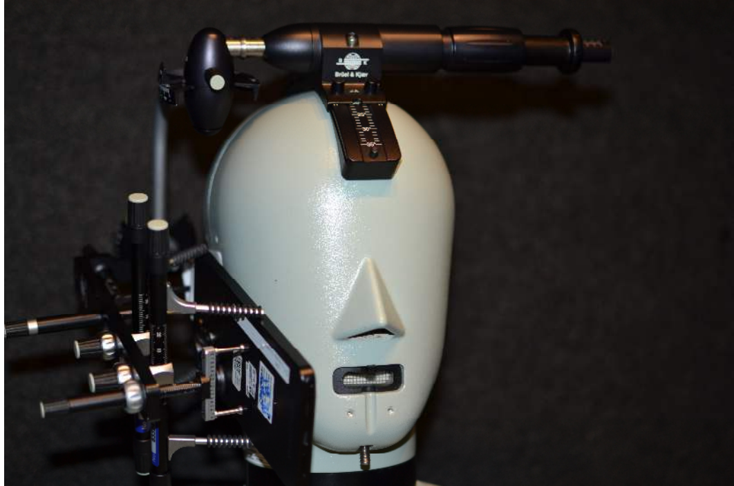
Figure 17-3 Test Setup for Wireless Device
