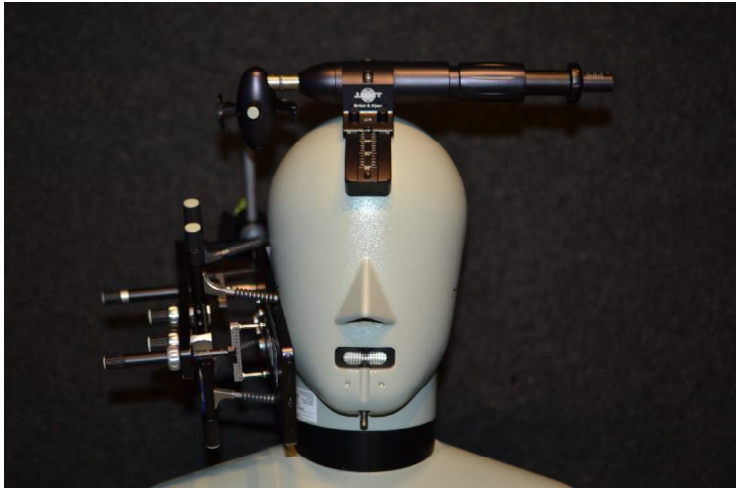
Figure 17-2 Test Setup for Wireless Device
