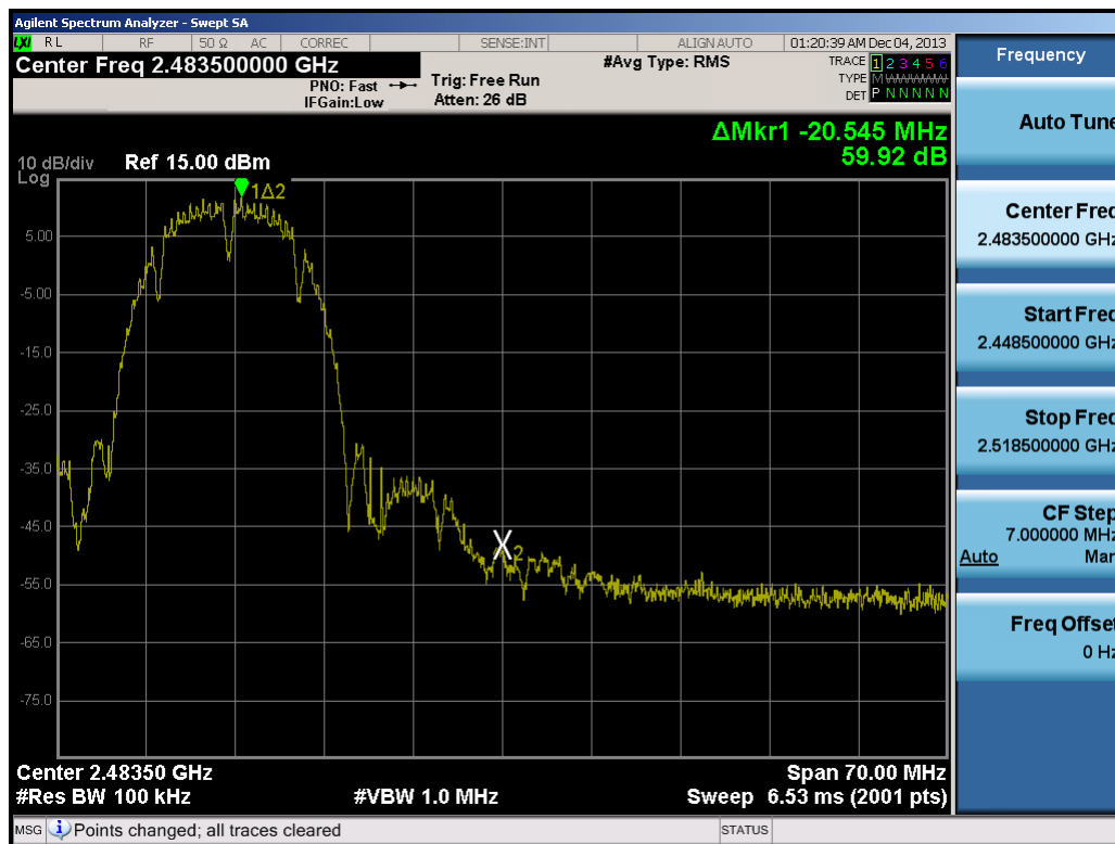
Plot 6-20. Band Edge Plot (802.11b – Ch. 11)
