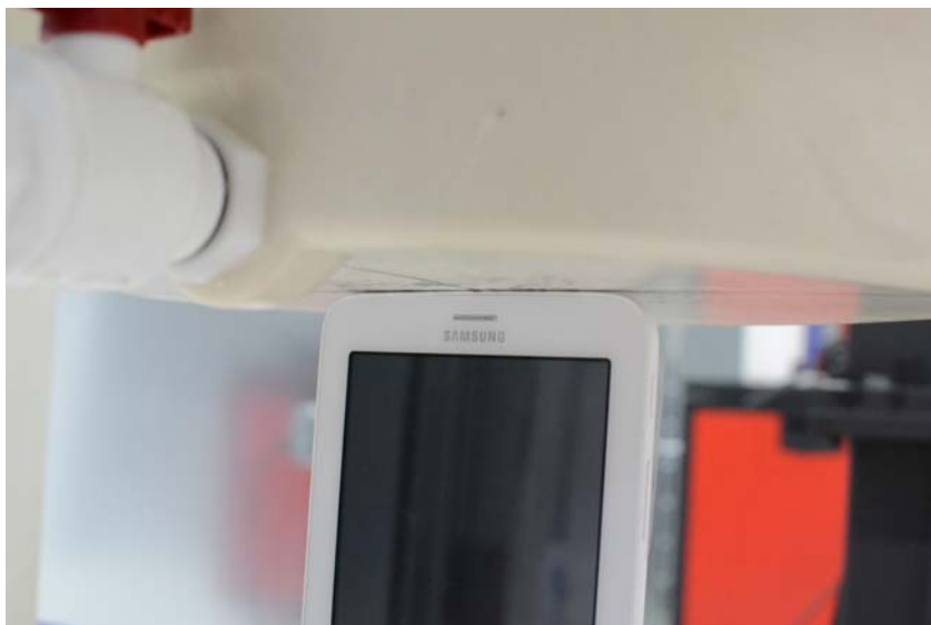
SAR Test Setup Photo 8 – Top Edge at 0.0 mm
