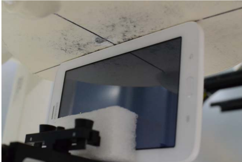
SAR Test Setup Photo 9 – Right Edge at 0.0 mm
