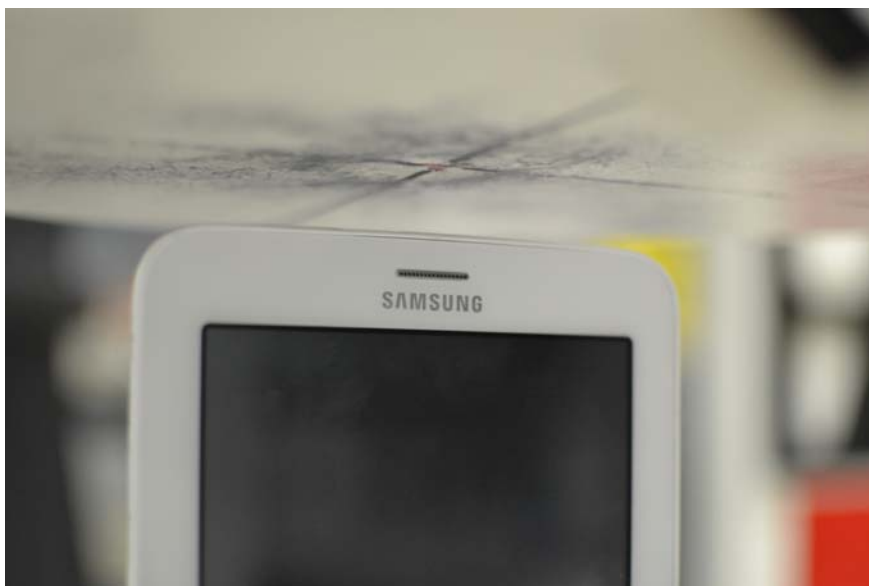
SAR Test Setup Photo 7 – Top Edge at 11.0 mm
