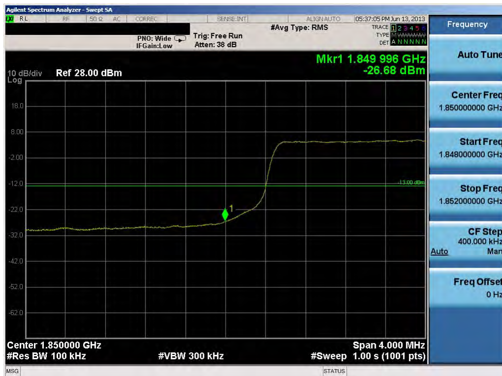
Plot 10-29. Lower Band Edge Plot (10.0MHz QPSK – RB Size 50)
