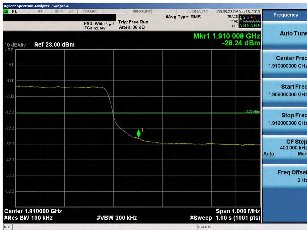
Plot 10-39. Upper Band Edge Plot (10.0MHz QPSK – RB Size 50)
