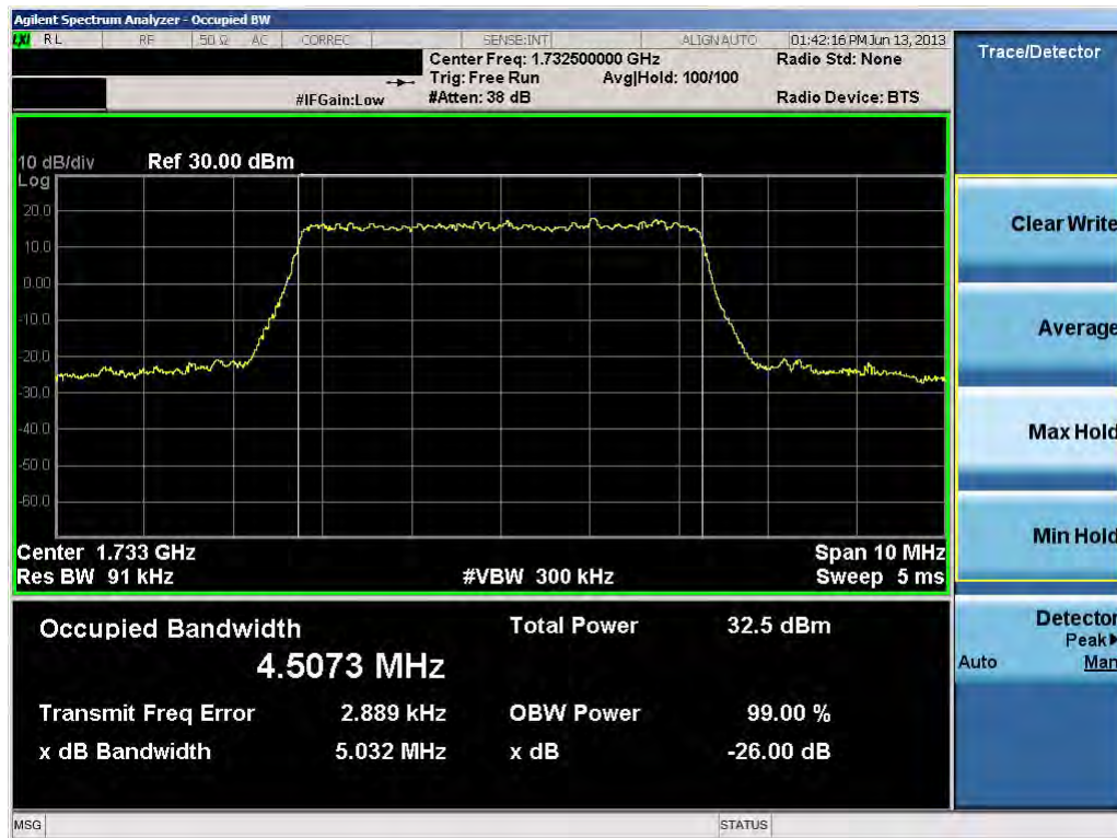
Plot 9-3. Occupied Bandwidth Plot (5.0MHz QPSK – RB Size 25)
