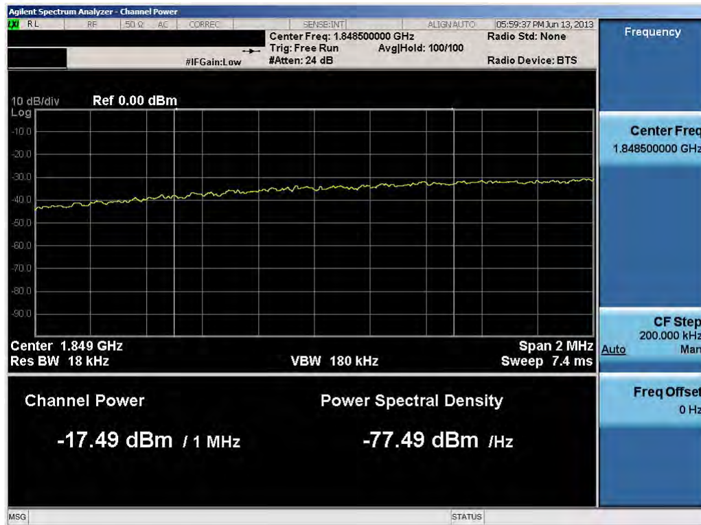
Plot 10-2. Lower Extended Band Edge Plot (3.0MHz QPSK – RB Size 15)
