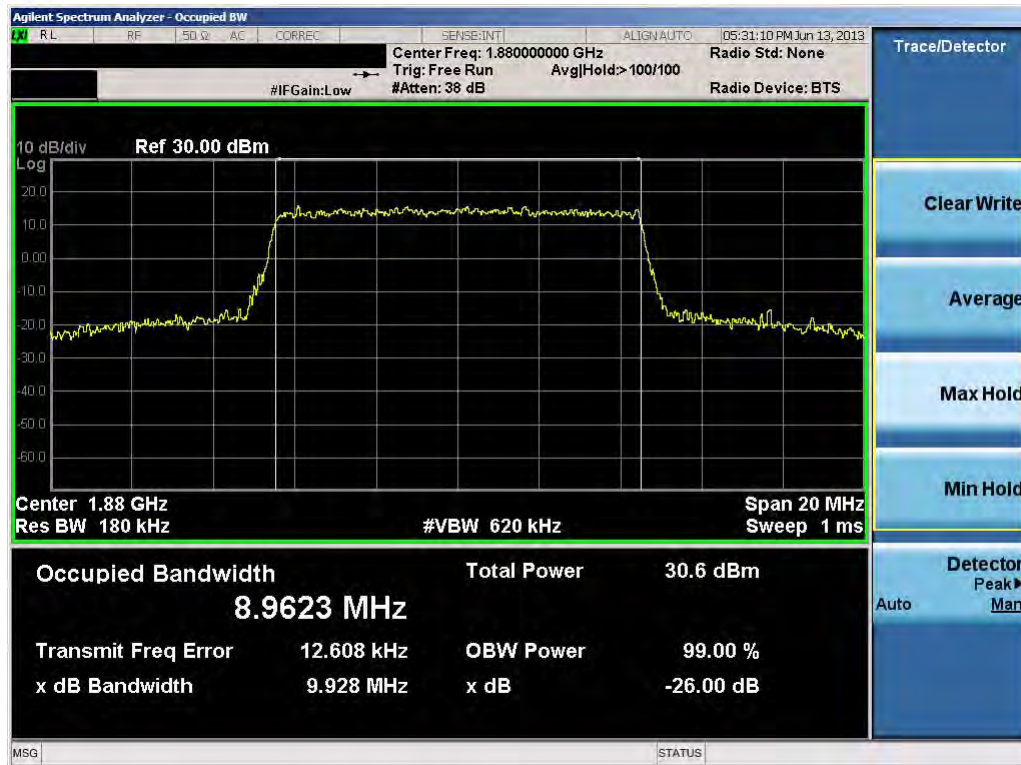
Plot 10-32. Occupied Bandwidth Plot (10.0MHz 16-QAM – RB Size 50)
