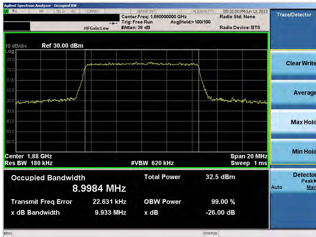
Plot 10-31. Occupied Bandwidth Plot (10.0MHz QPSK – RB Size 50)
