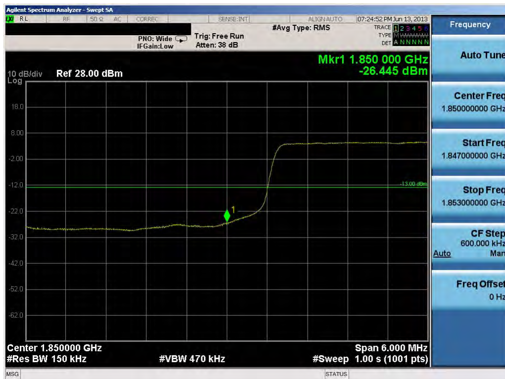
Plot 10-43. Lower Band Edge Plot (15.0MHz QPSK – RB Size 75)
