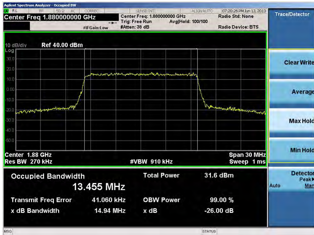
Plot 10-46. Occupied Bandwidth Plot (15.0MHz 16-QAM – RB Size 75)
