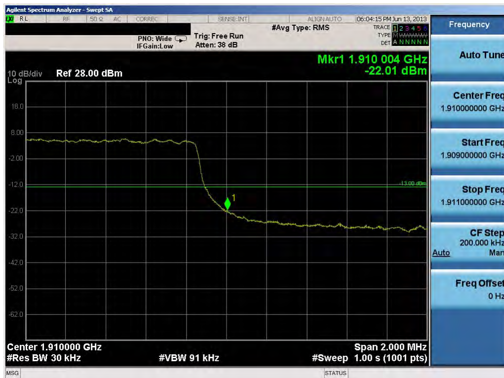
Plot 10-11. Upper Band Edge Plot (3.0MHz QPSK – RB Size 15)
