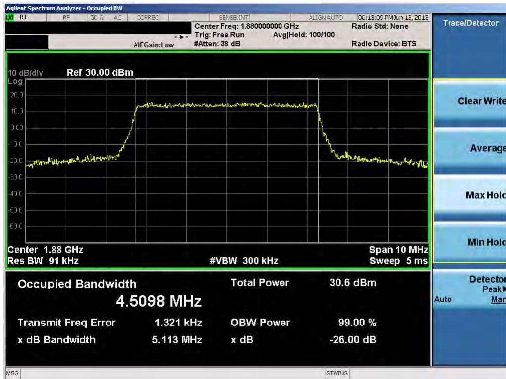
Plot 10-18. Occupied Bandwidth Plot (5.0MHz 16-QAM – RB Size 25)
