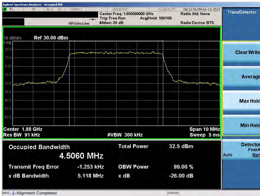
Plot 10-17. Occupied Bandwidth Plot (5.0MHz QPSK – RB Size 25)
