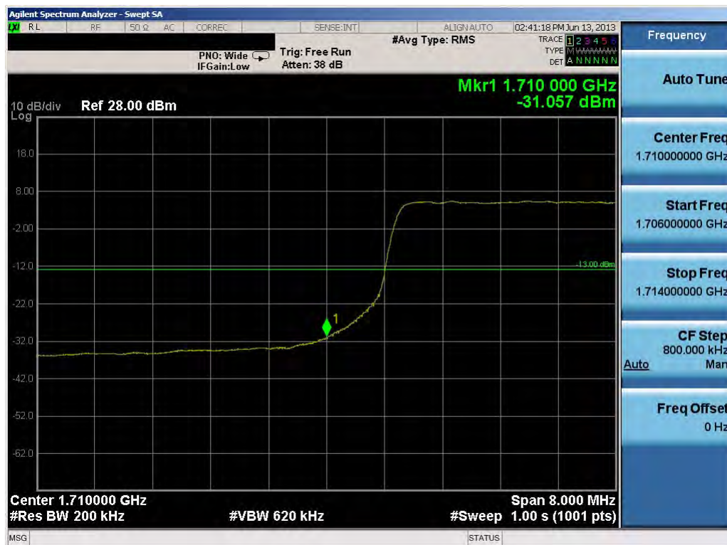
Plot 9-43. Lower Band Edge Plot (20.0MHz QPSK – RB Size 100)
