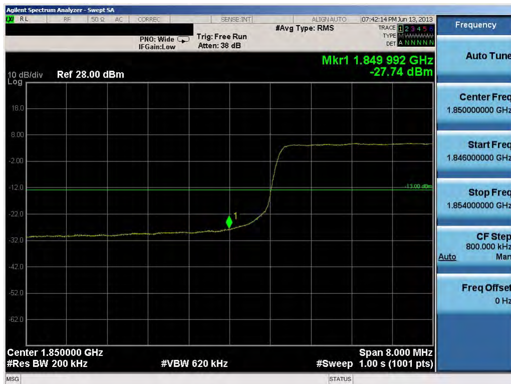
Plot 10-57. Lower Band Edge Plot (20.0MHz QPSK – RB Size 100)
