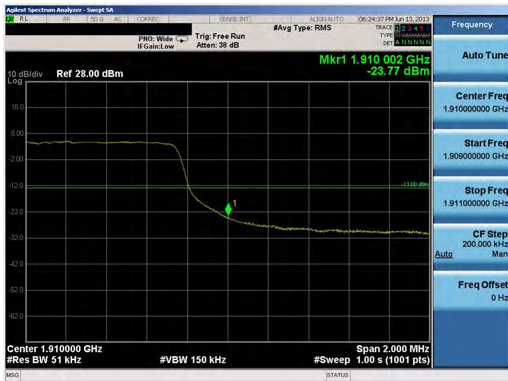
Plot 10-25. Upper Band Edge Plot (5.0MHz QPSK – RB Size 25)
