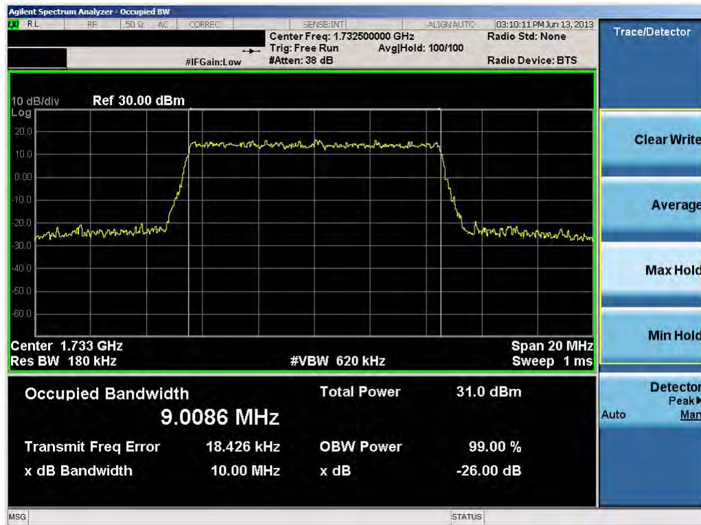
Plot 9-18. Occupied Bandwidth Plot (10.0MHz 16-QAM – RB Size 50)
