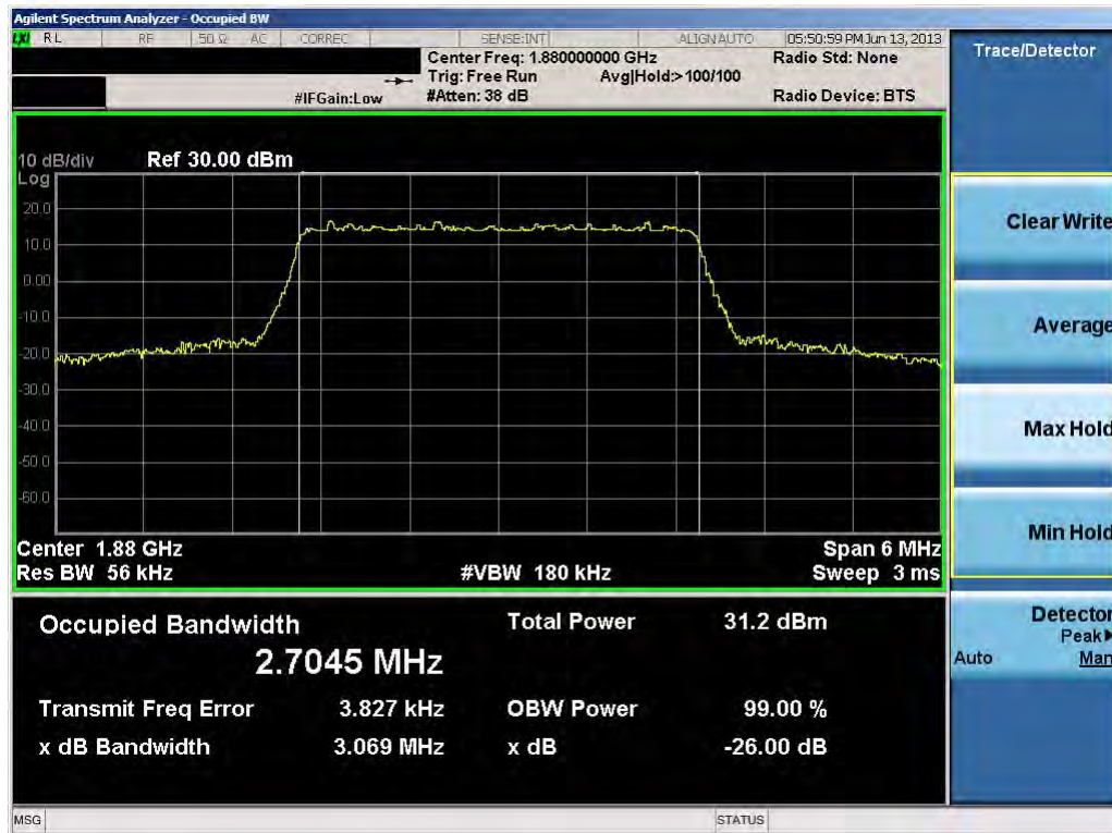
Plot 10-4. Occupied Bandwidth Plot (3.0MHz 16-QAM – RB Size 15)
