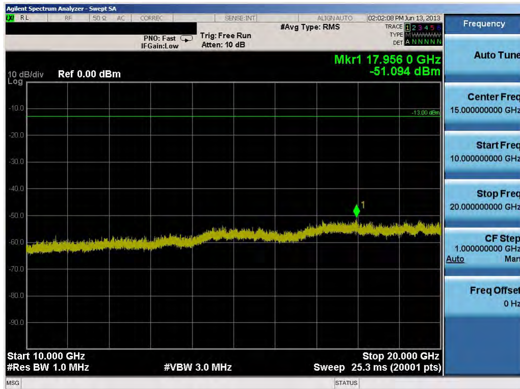
Plot 9-36. Conducted Spurious Plot (15.0MHz QPSK – RB Size 1, RB Offset 0 – Mid Channel)
