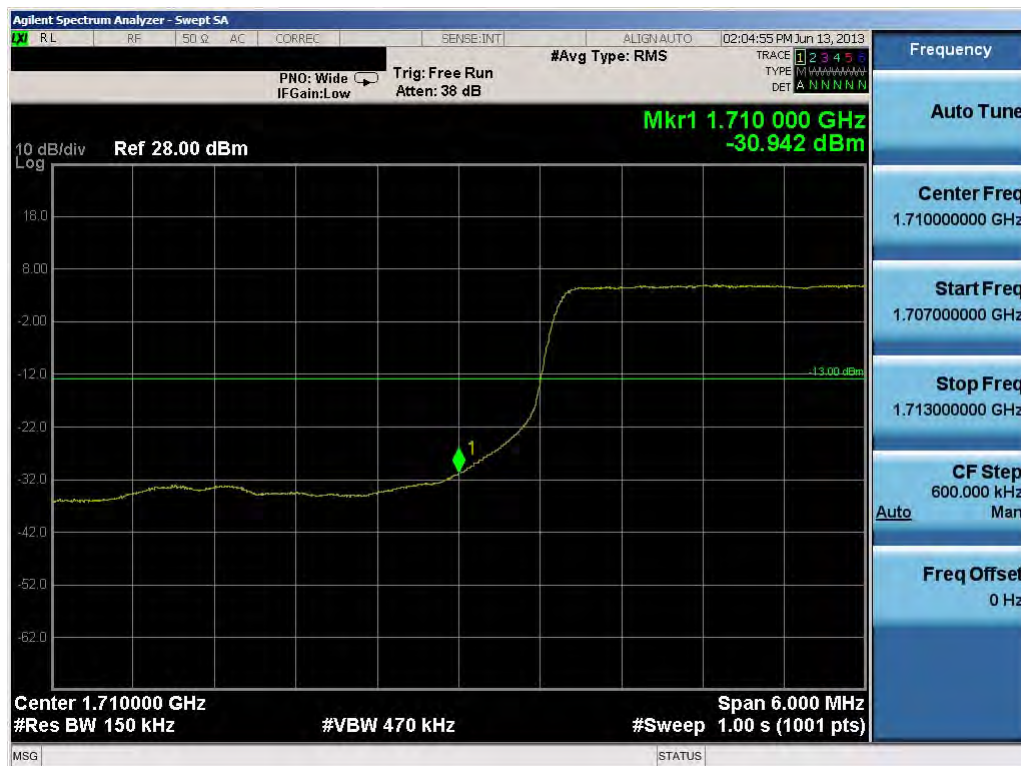
Plot 9-29. Lower Band Edge Plot (15.0MHz QPSK – RB Size 75)
