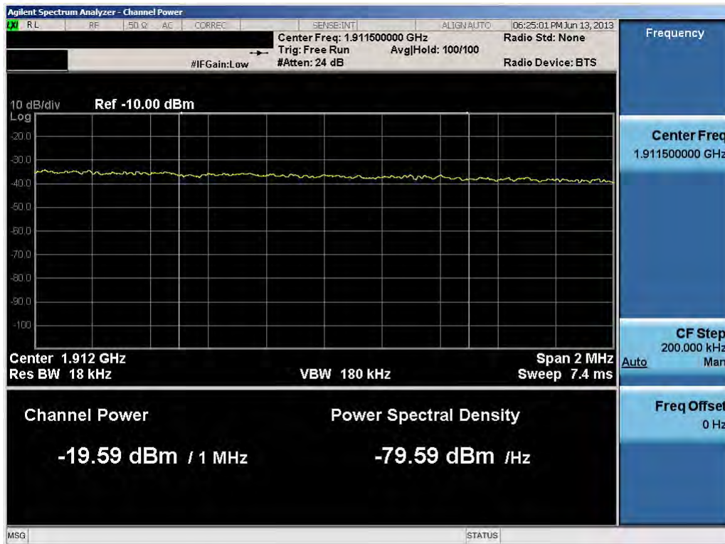
Plot 10-26. Upper Extended Band Edge Plot (5.0MHz QPSK – RB Size 25)
