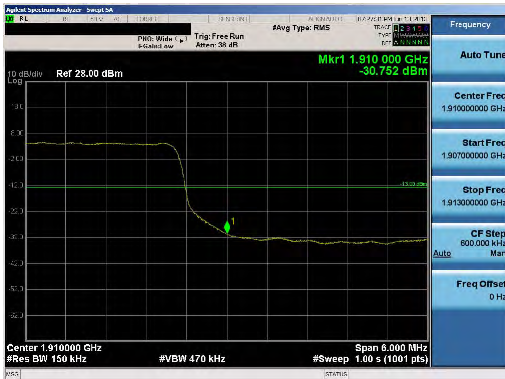
Plot 10-53. Upper Band Edge Plot (15.0MHz QPSK – RB Size 75)
