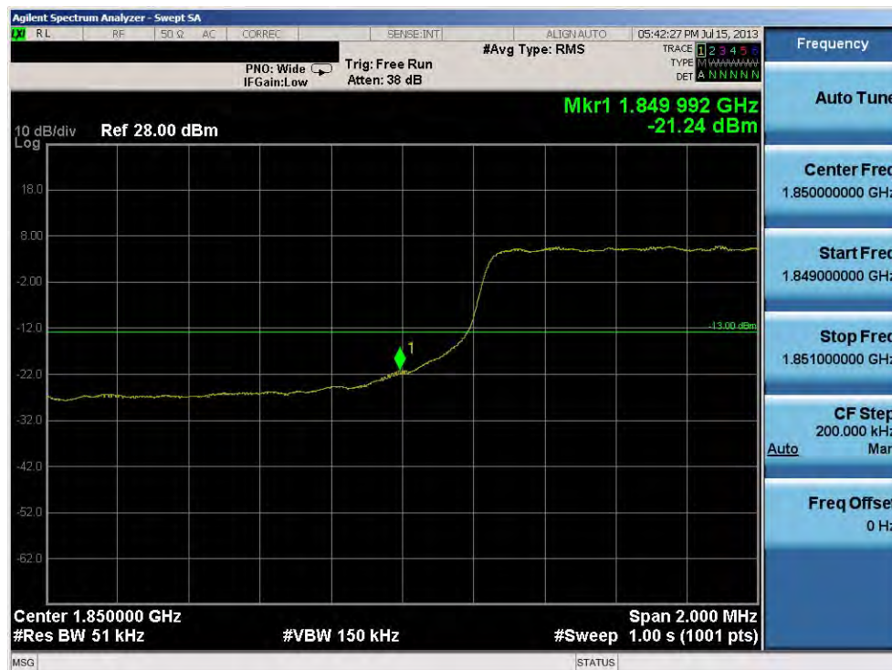
Plot 10-15. Lower Band Edge Plot (5.0MHz QPSK – RB Size 25)
