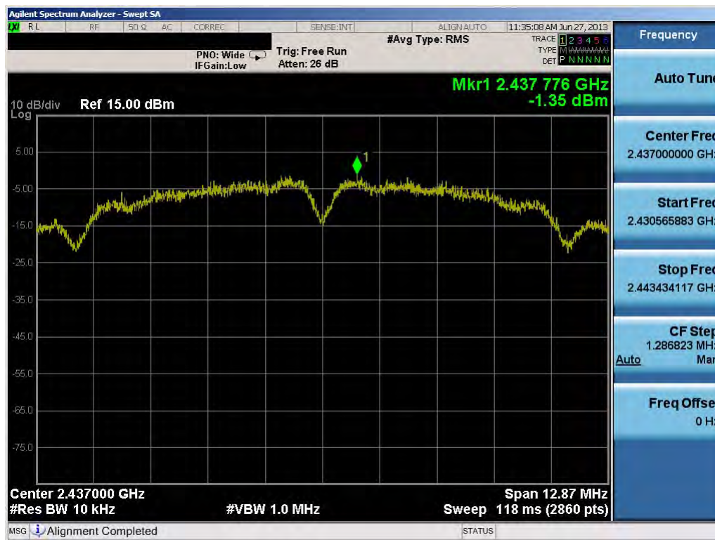
Plot 6-19. Power Spectral Density Plot (802.11b - Ch. 6)
