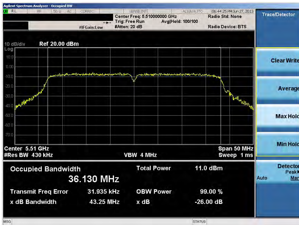
Plot 6-23. 26dB Bandwidth Plot (40MHz BW 802.11n (UNII Band 3) – Ch. 102)
