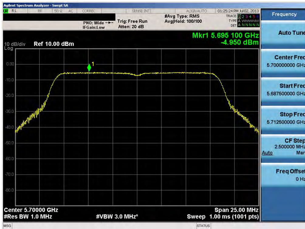
Plot 6-44. Peak Power Spectral Density Plot (802.11a (UNII Band 3) – Ch. 140)
