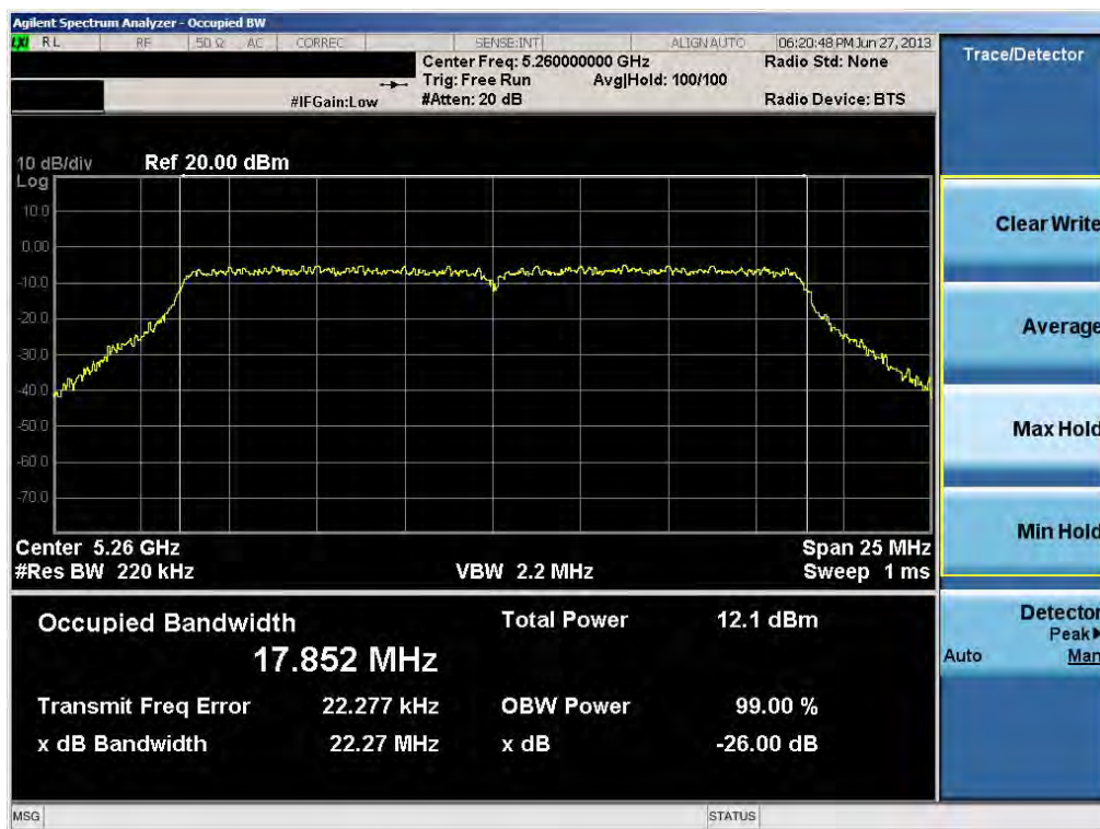
Plot 6-12. 26dB Bandwidth Plot (20MHz BW 802.11n (UNII Band 2) – Ch. 52)
