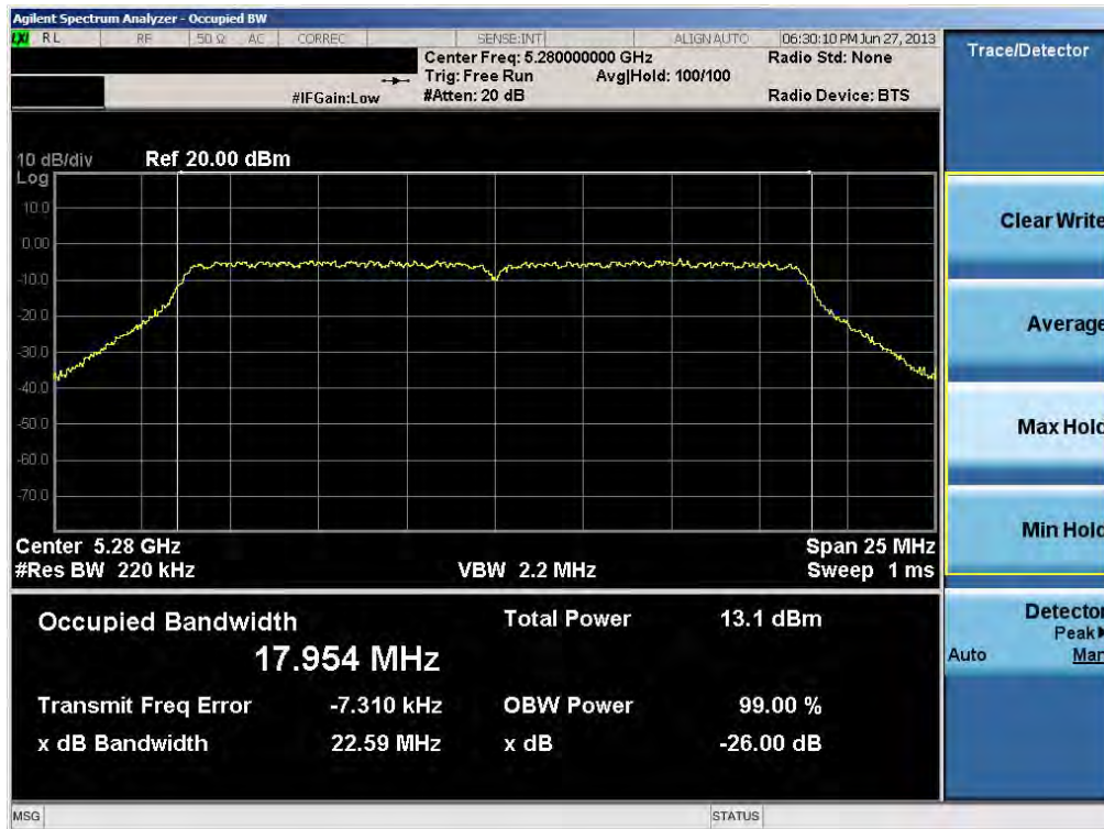
Plot 6-13. 26dB Bandwidth Plot (20MHz BW 802.11n (UNII Band 2) – Ch. 56)
