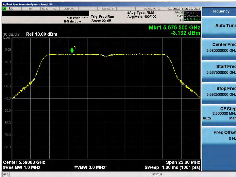
Plot 6-43. Peak Power Spectral Density Plot (802.11a (UNII Band 3) – Ch. 116)
