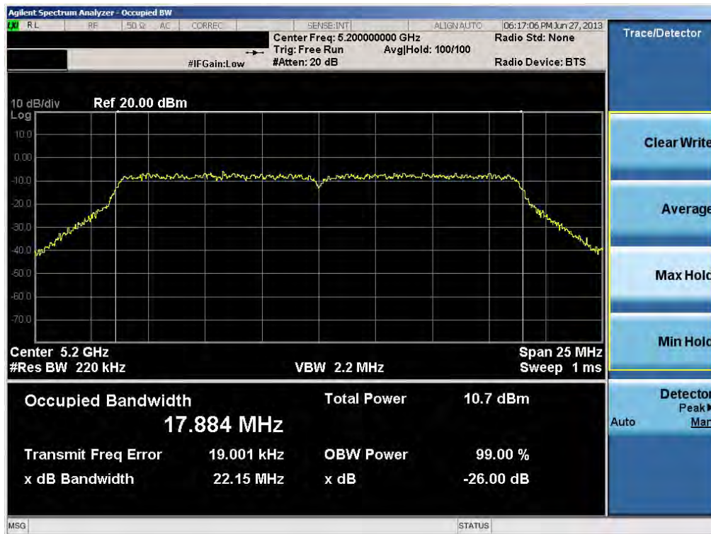
Plot 6-5. 26dB Bandwidth Plot (20MHz BW 802.11n (UNII Band 1) – Ch. 40)
