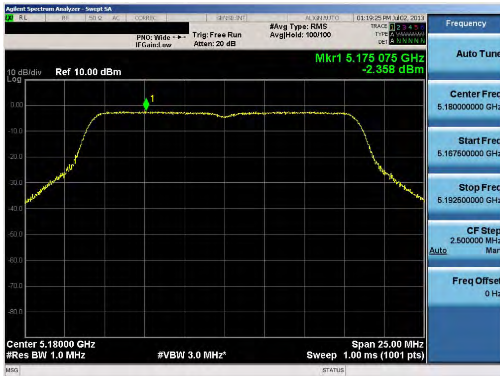
Plot 6-26. Peak Power Spectral Density Plot (802.11a (UNII Band 1) – Ch. 36)
