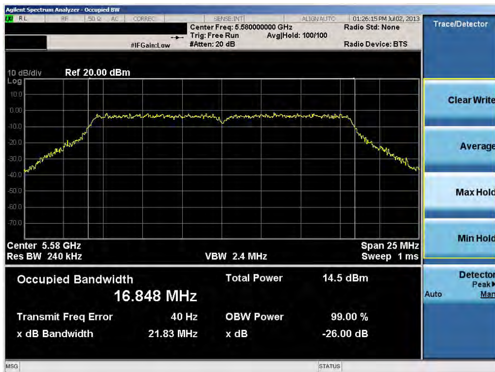
Plot 6-18. 26dB Bandwidth Plot (802.11a (UNII Band 3) – Ch. 116)
