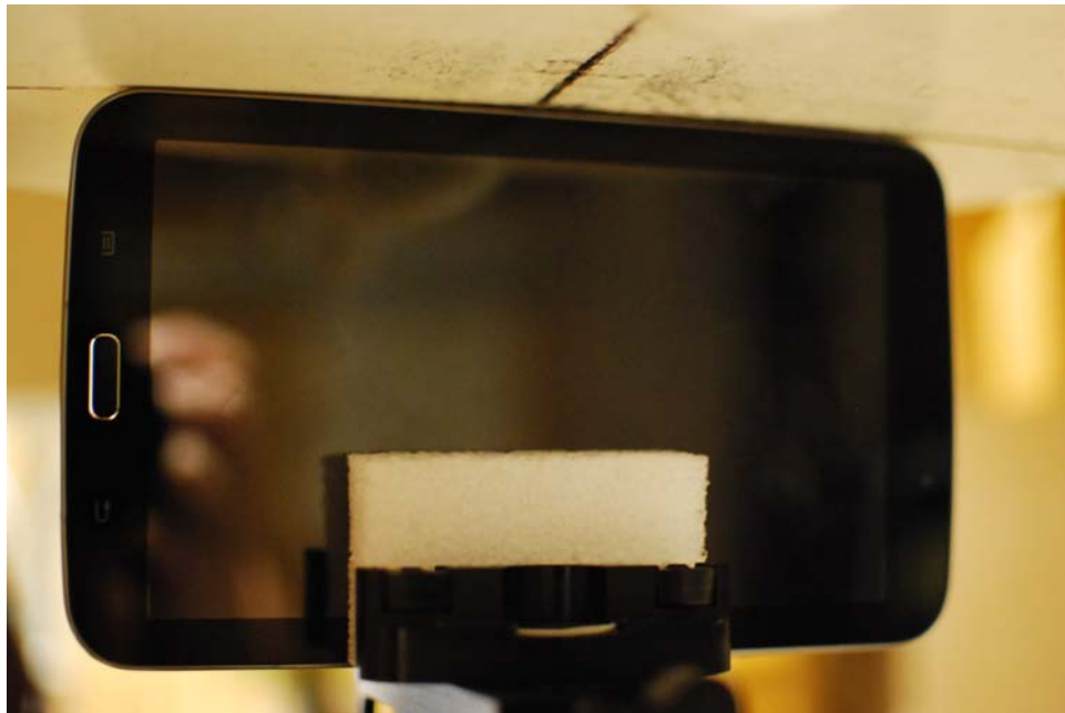
SAR Test Setup Photo 6: Left at 0.0 cm
