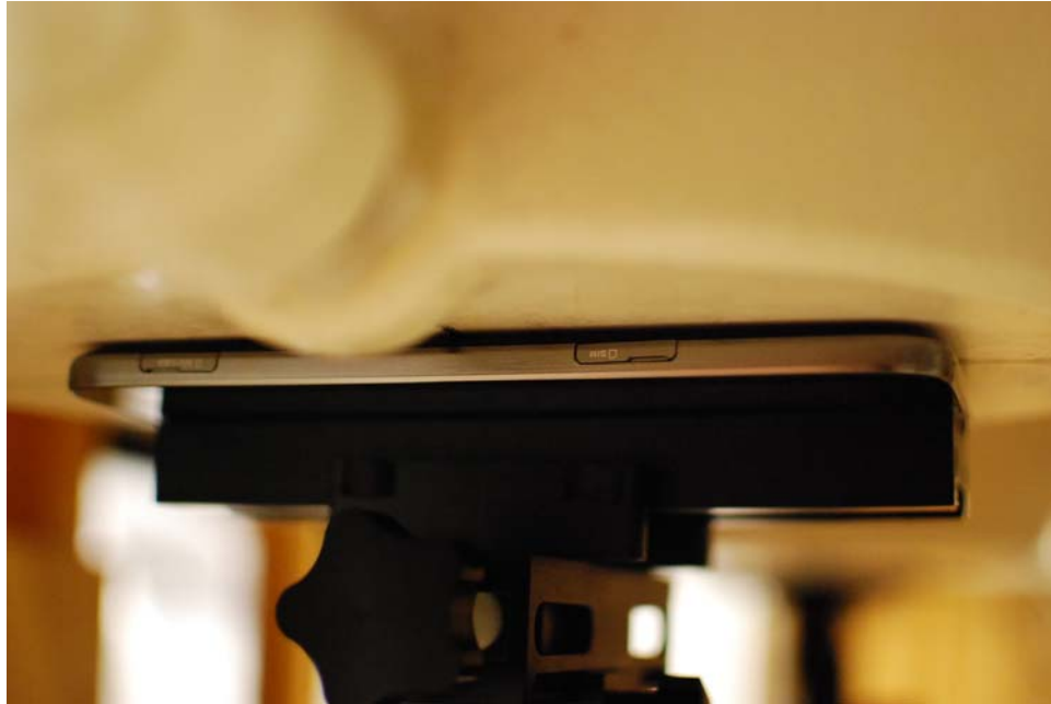
SAR Test Setup Photo 1: Back at 0.0 cm
