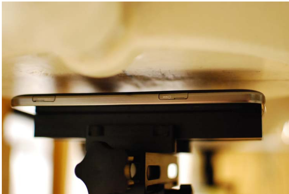
SAR Test Setup Photo 2: Back at 1.4 cm
