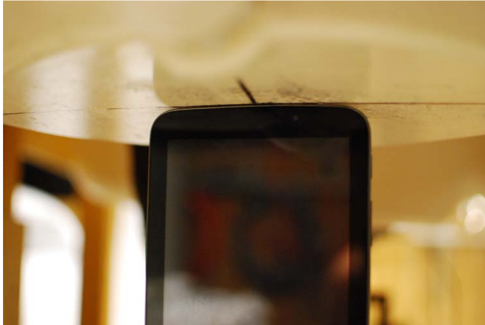
SAR Test Setup Photo 3: Top at 0.0 cm
