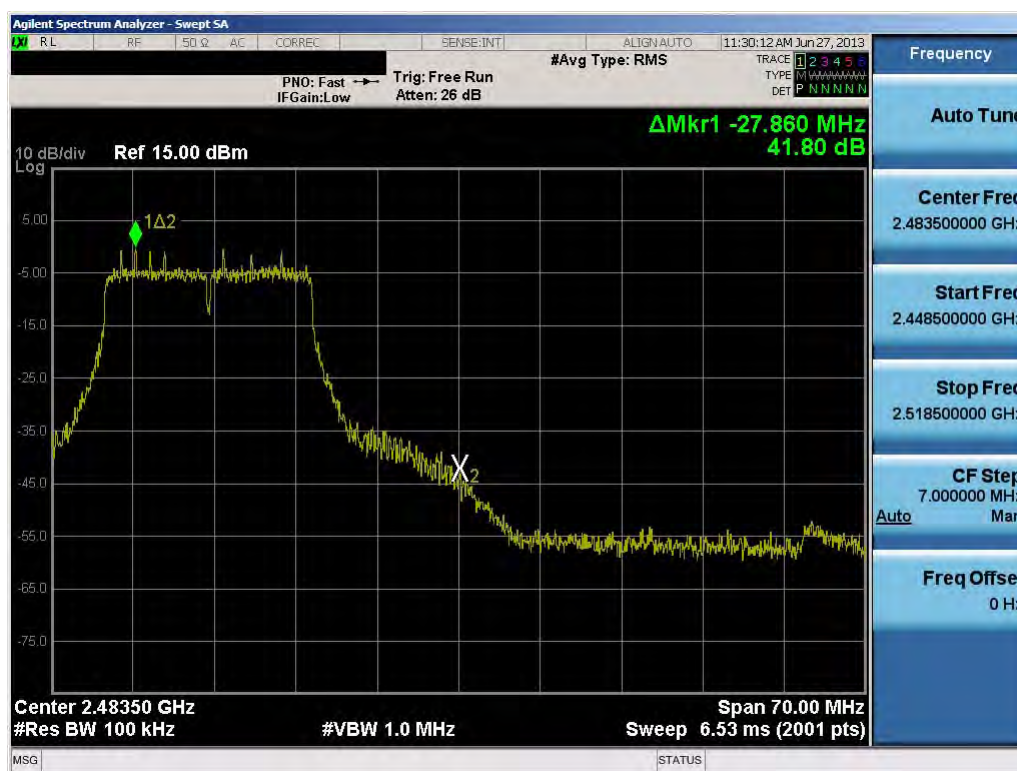
Plot 6-40. Band Edge Plot (802.11n (2.4GHz) – Ch. 11)
