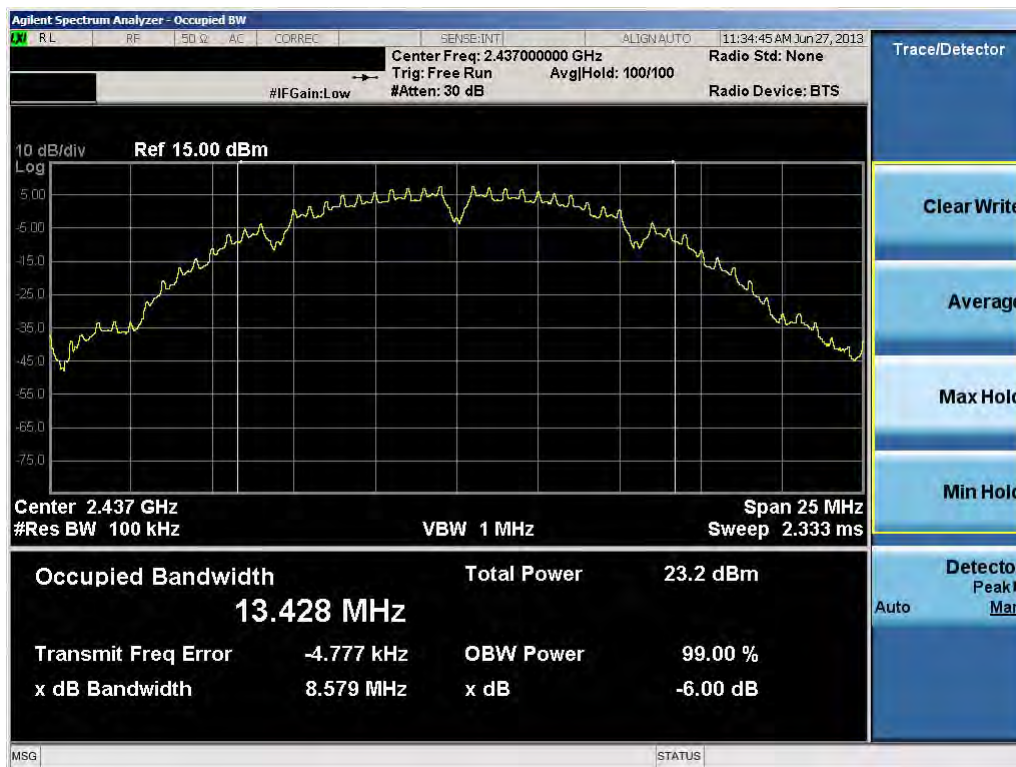
Plot 6-2. 6dB Bandwidth Plot (802.11b – Ch. 6)
