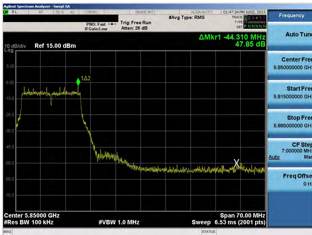
Plot 6-42. Band Edge Plot (802.11a – Ch. 165)
