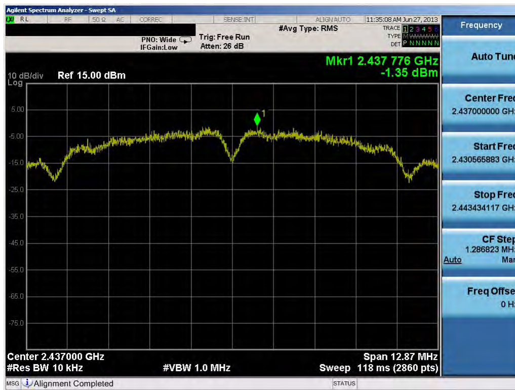
Plot 6-19. Power Spectral Density Plot (802.11b - Ch. 6)
