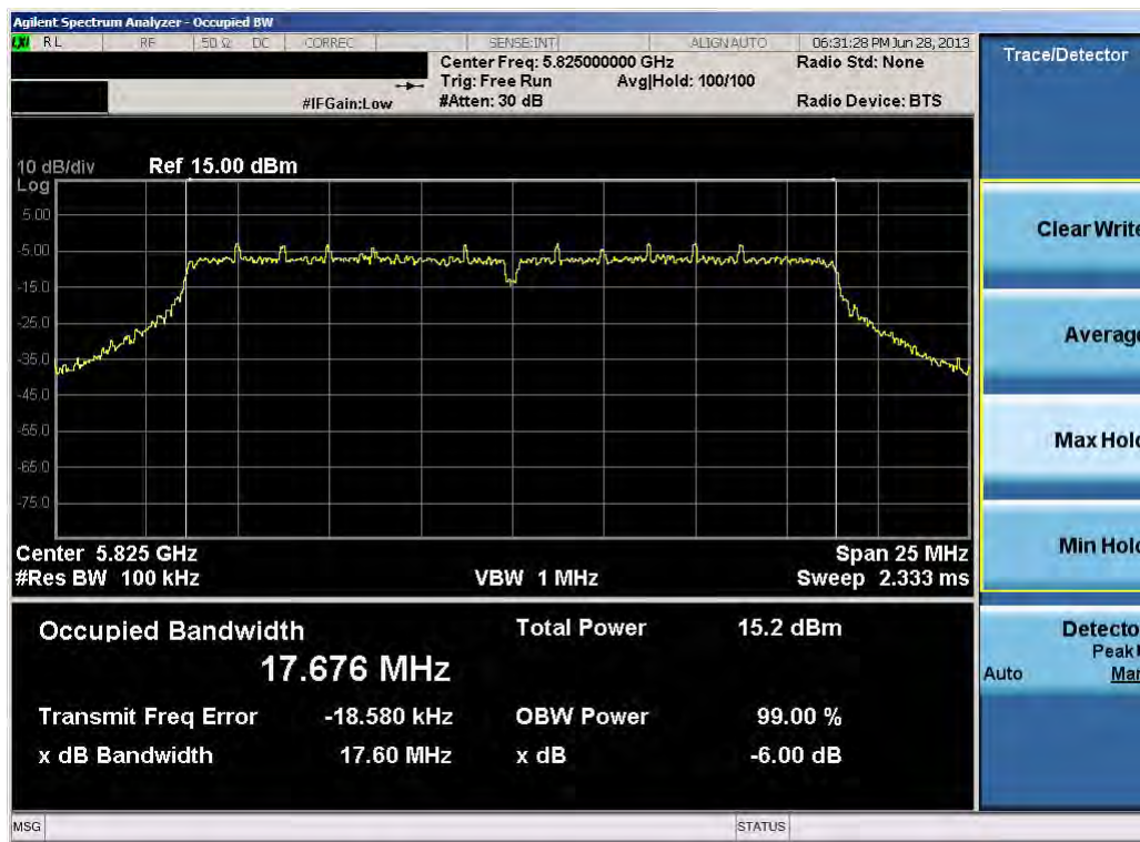
Plot 6-15. 6dB Bandwidth Plot (20MHz BW 802.11n (5.8GHz) – Ch. 165)
