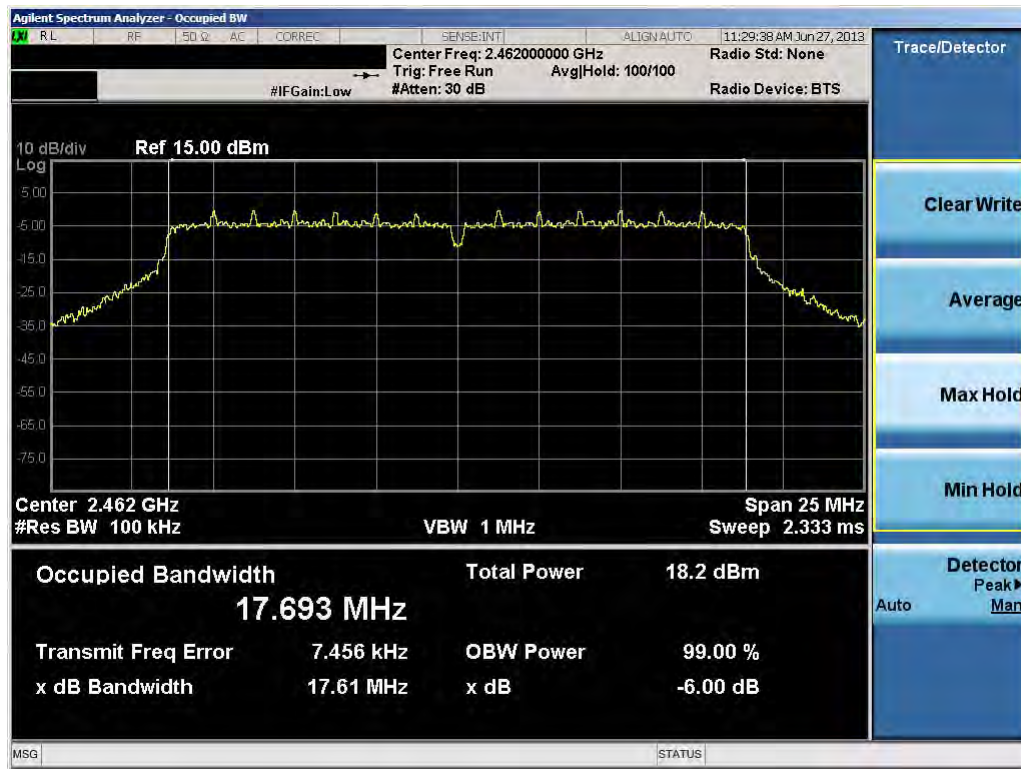
Plot 6-9. 6dB Bandwidth Plot (802.11n (2.4GHz) – Ch. 11)
