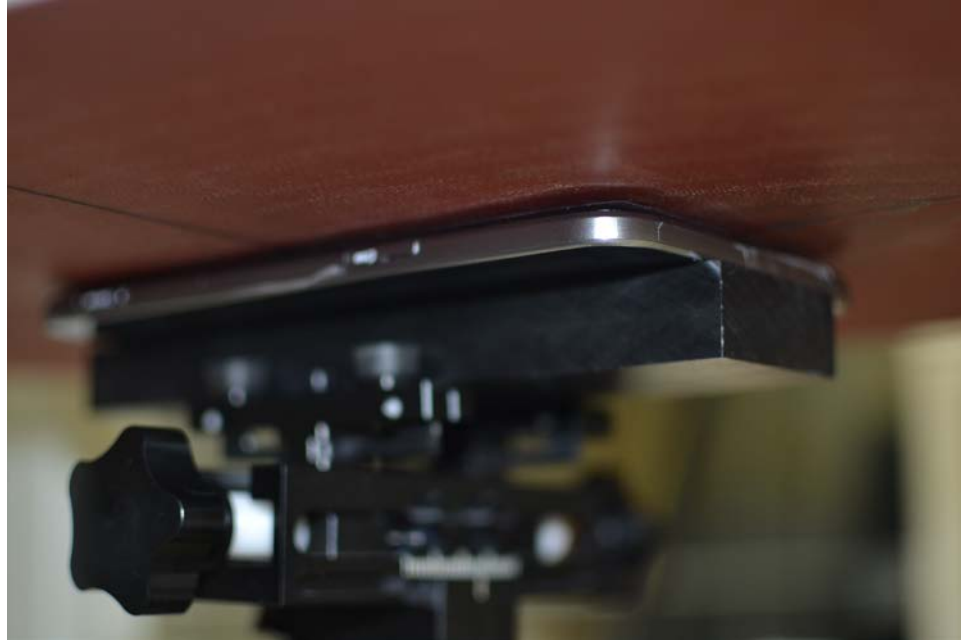
SAR Test Setup Photo 1: Back at 0.0 cm
