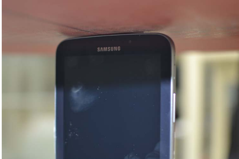
SAR Test Setup Photo 3: Top at 0.0 cm
