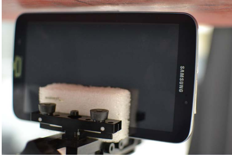
SAR Test Setup Photo 7: Left at 0.4 cm
