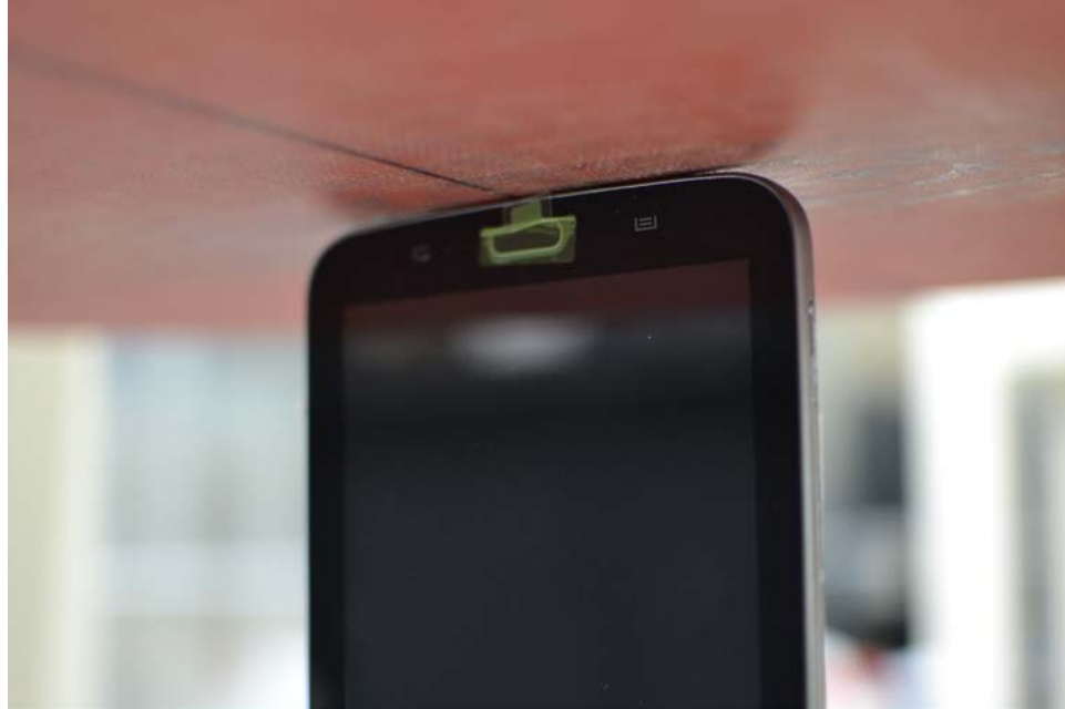
SAR Test Setup Photo 5: Bottom at 0.0 cm
