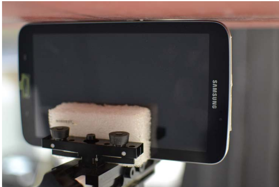
SAR Test Setup Photo 6: Left at 0.0 cm
