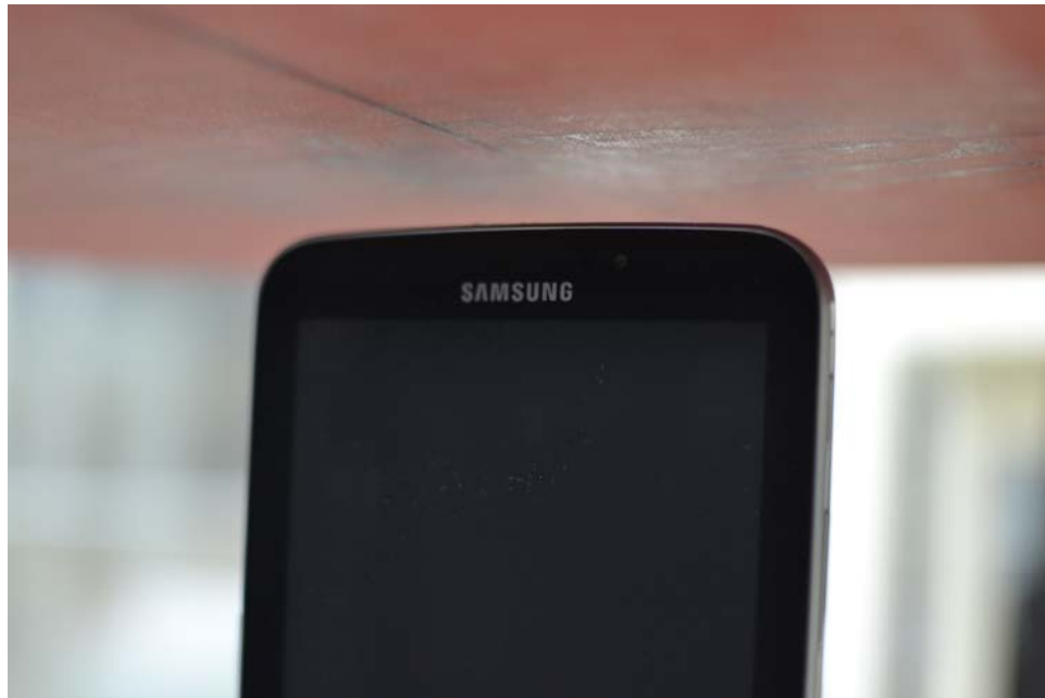
SAR Test Setup Photo 4: Top at 1.4 cm
