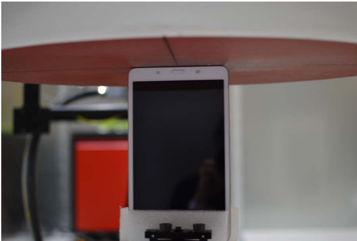
SAR Test Setup Photo 2: Bottom at 0.0 cm
