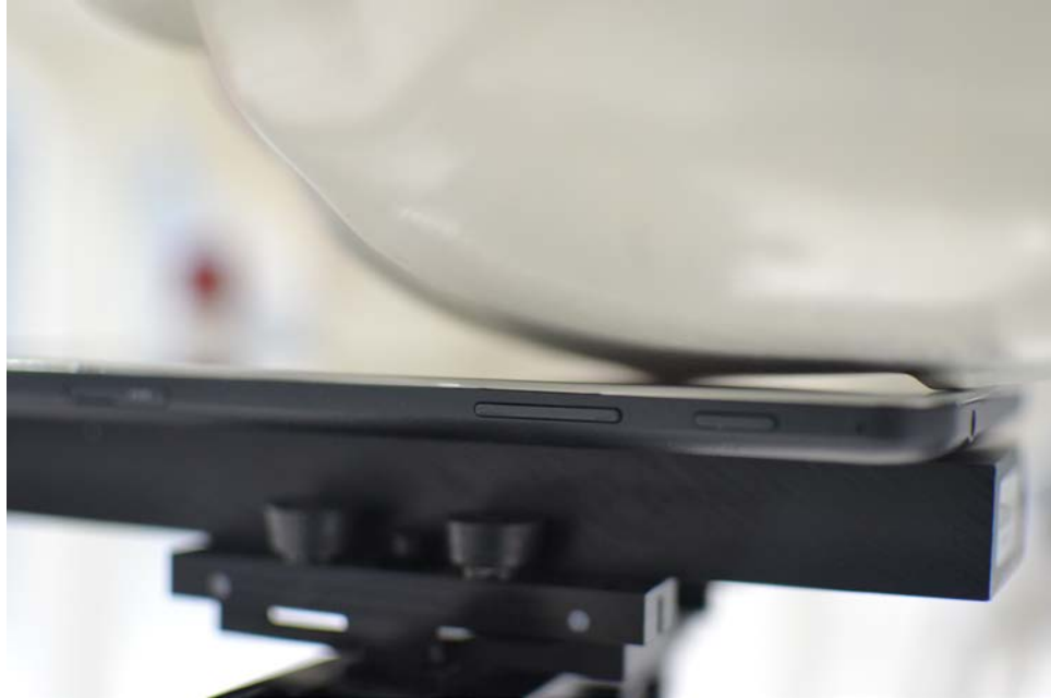
SAR Test Setup Photo 3: Left Cheek
