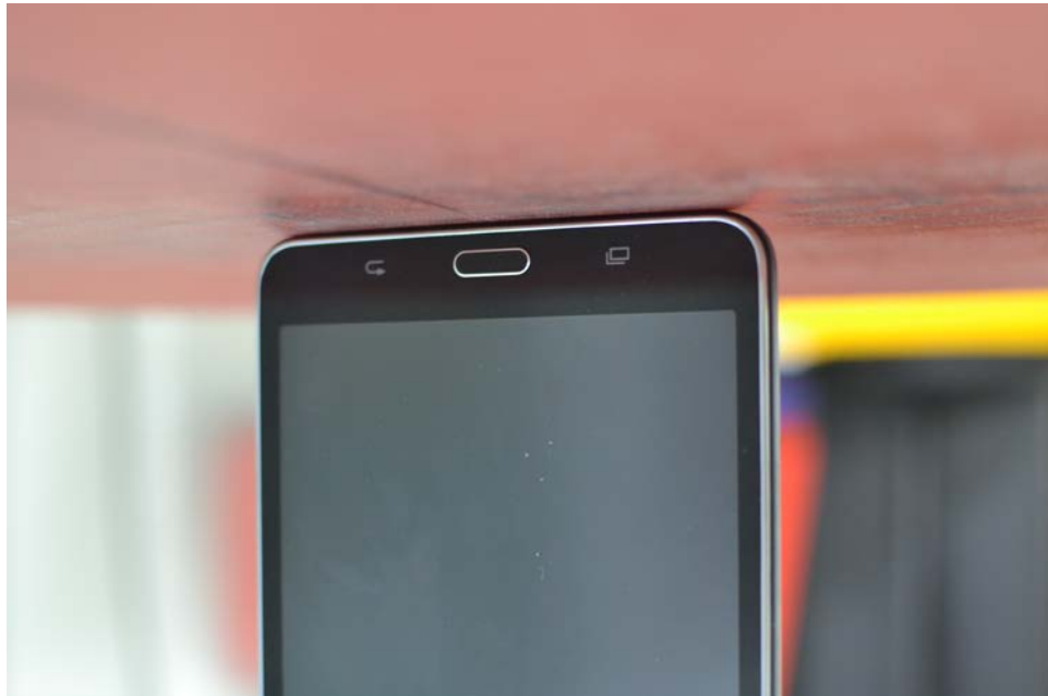
SAR Test Setup Photo 10: Bottom at 0.0 cm
