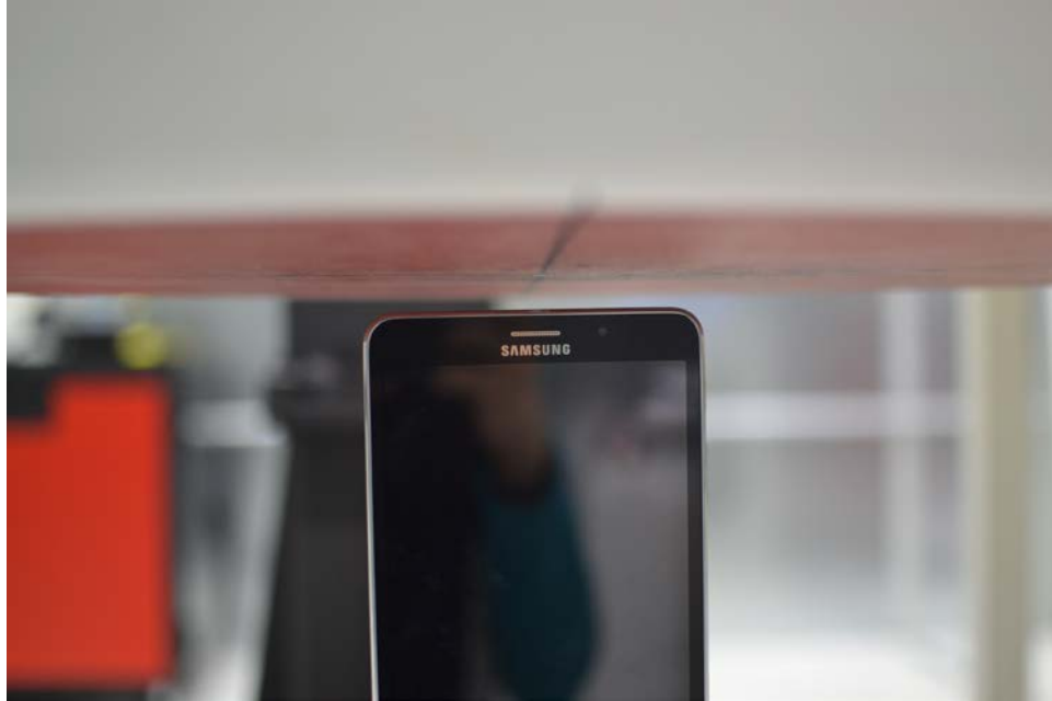
SAR Test Setup Photo 7: Top Edge at 1.1 cm
