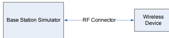
Figure 8-2 Power Measurement Setup
