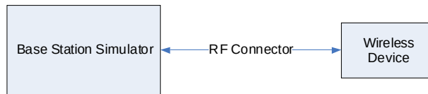
Figure 9-1 Power Measurement Setup
