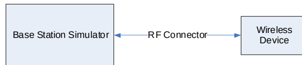
Figure 9-2 Power Measurement Setup
