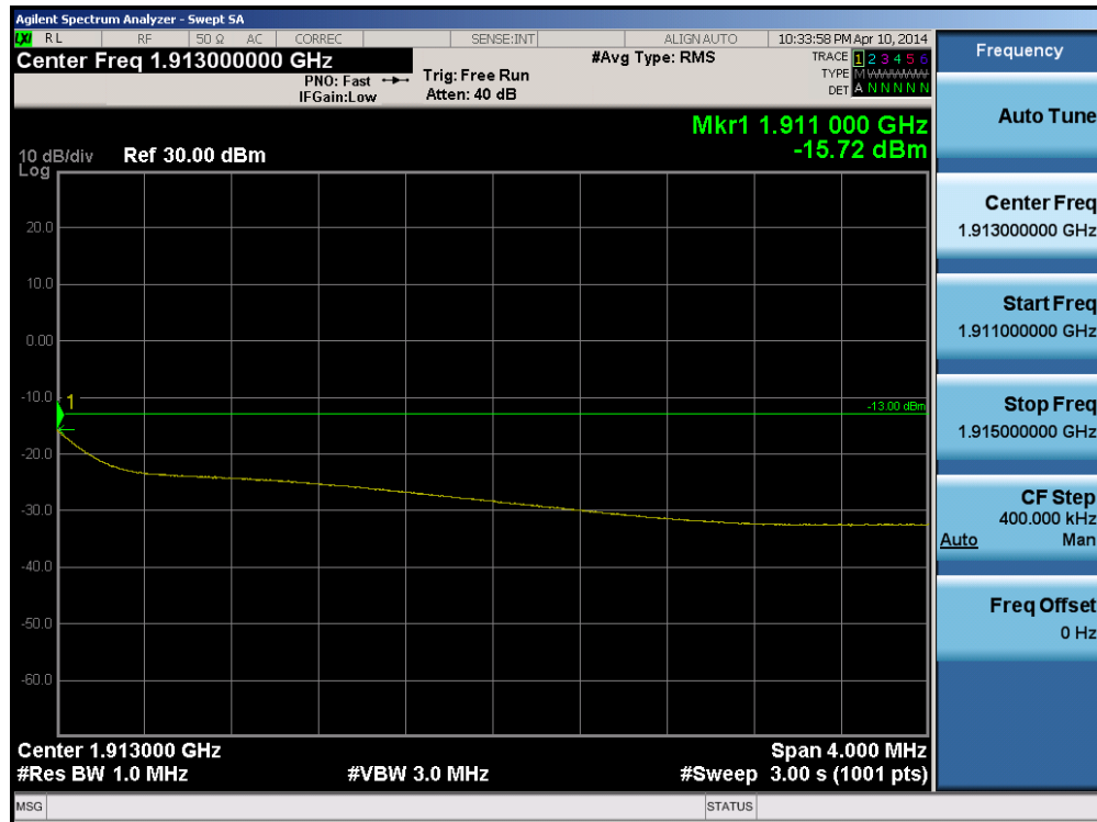
Plot 6-34. 4MHz Span Plot (PCS WCDMA Mode – Ch. 9538)
