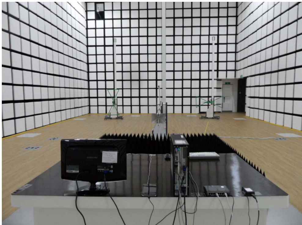
[ Radiated Disturbance for Above 1 GHz – Rear ]
