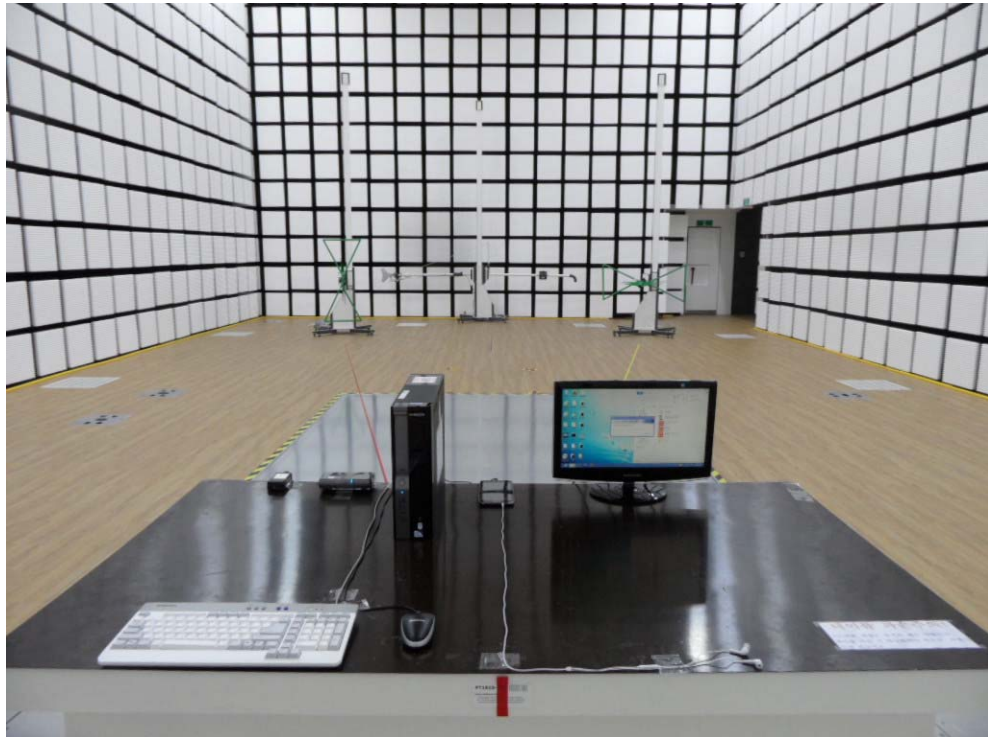
[ Radiated Disturbance for Below 1 GHz – Front ]
