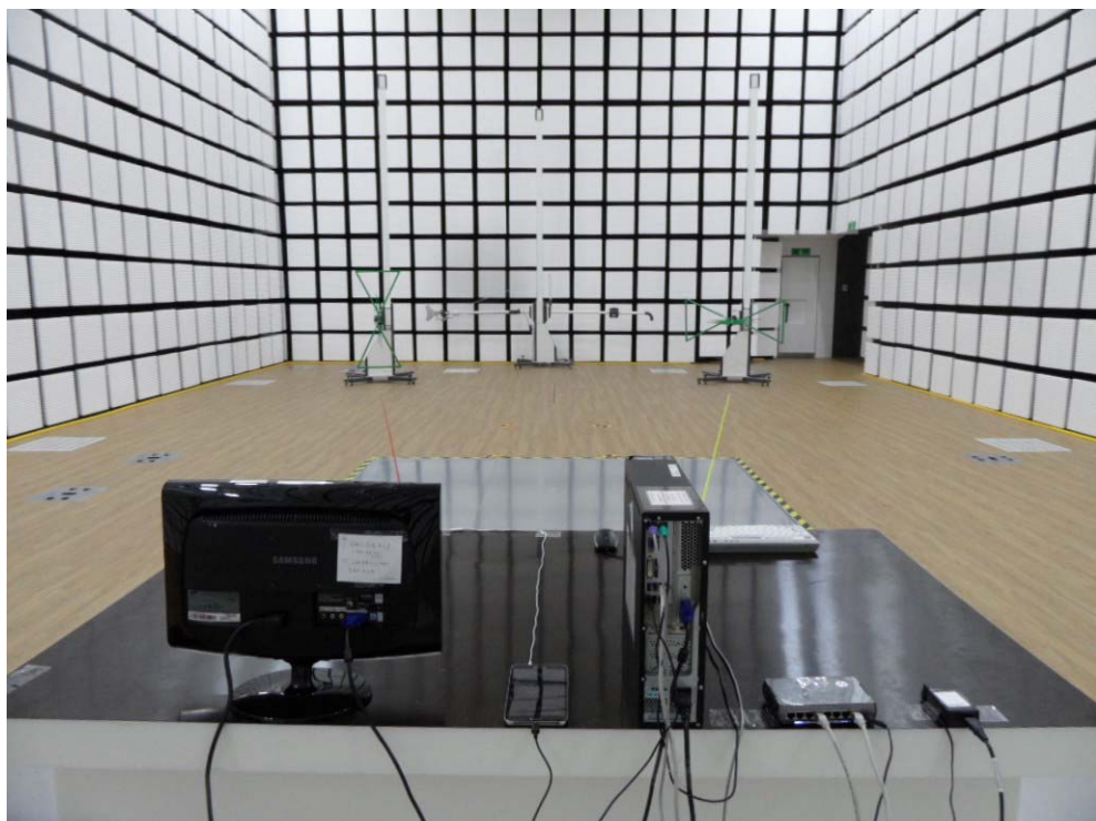
[ Radiated Disturbance for Below 1 GHz – Rear ]
