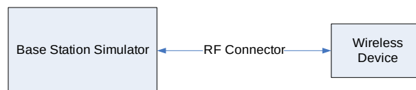
Figure 8-2 Power Measurement Setup
