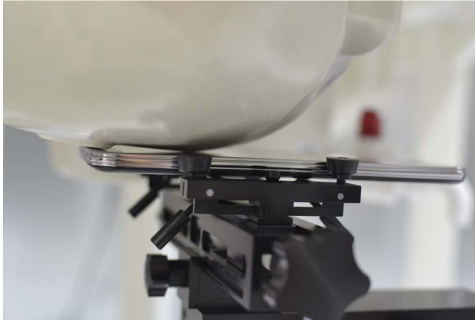
SAR Test Setup Photo 1- Right Cheek
