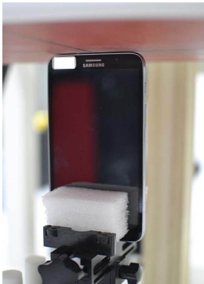
SAR Test Setup Photo 7- Top Edge at 0 mm
