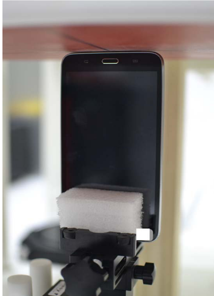
SAR Test Setup Photo 9- Bottom Edge at 0 mm
