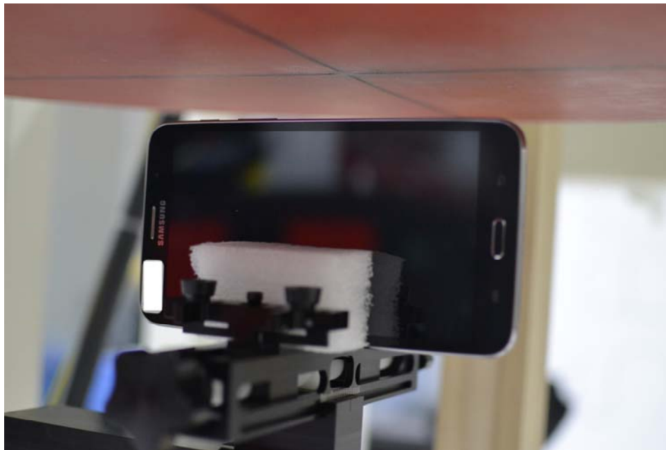
SAR Test Setup Photo 12- Right Edge at 15 mm
