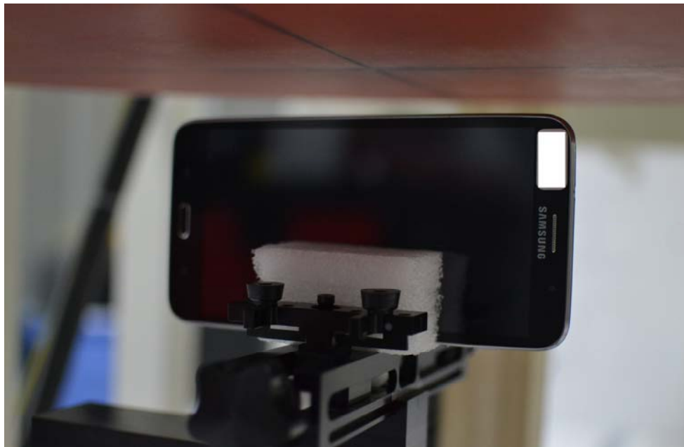
SAR Test Setup Photo 14- Left Edge at 15 mm
