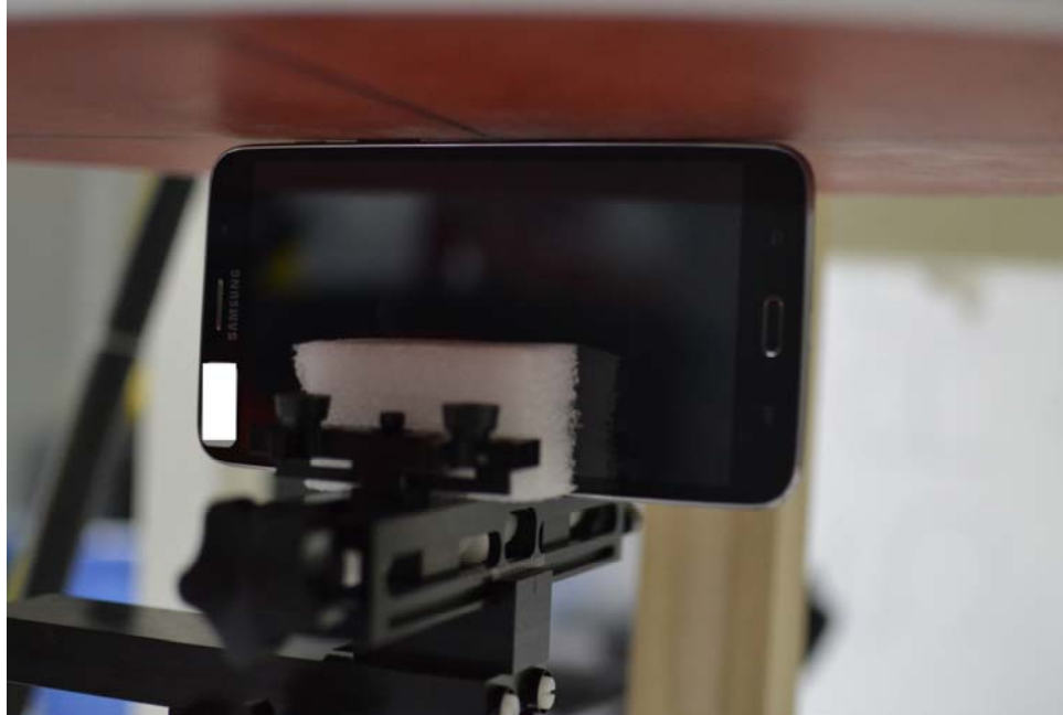
SAR Test Setup Photo 11- Right Edge at 0 mm
