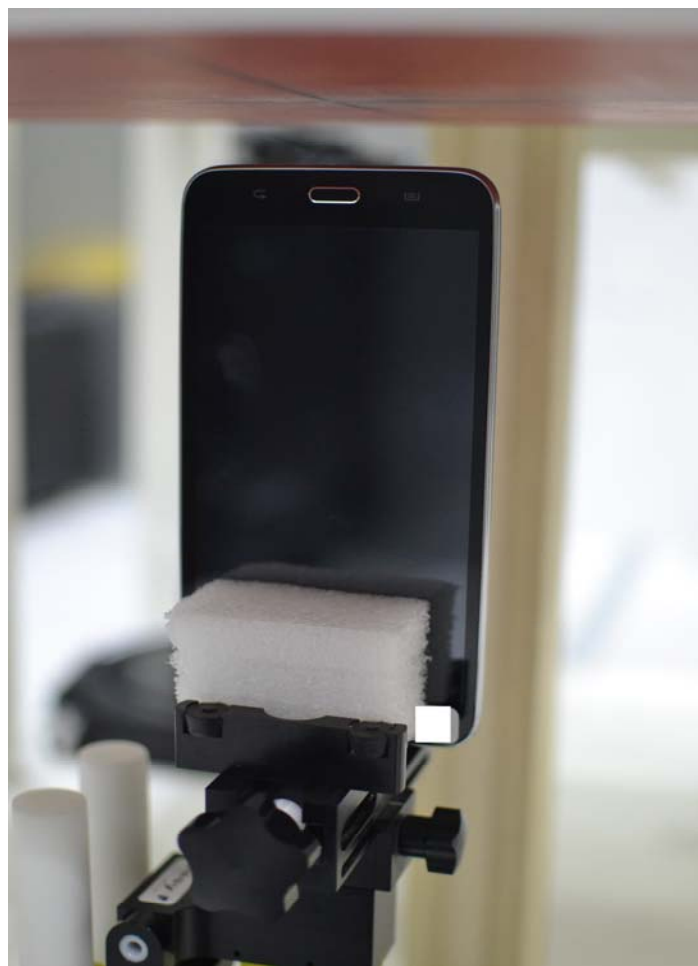
SAR Test Setup Photo 10- Bottom Edge at 10 mm
