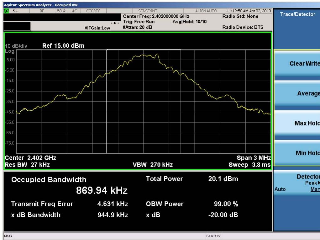
Plot 6-1. 20dB Bandwidth Plot (Bluetooth, 1Mbps – Ch. 0)
