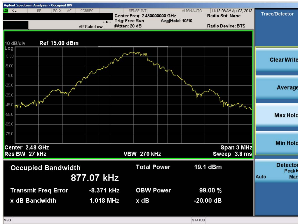
Plot 6-3. 20dB Bandwidth Plot (Bluetooth, 1Mbps – Ch. 78)
