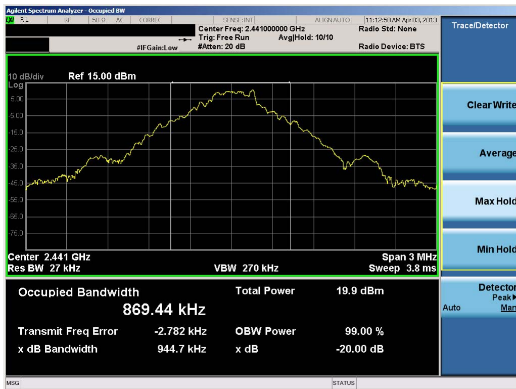
Plot 6-2. 20dB Bandwidth Plot (Bluetooth, 1Mbps – Ch. 39)
